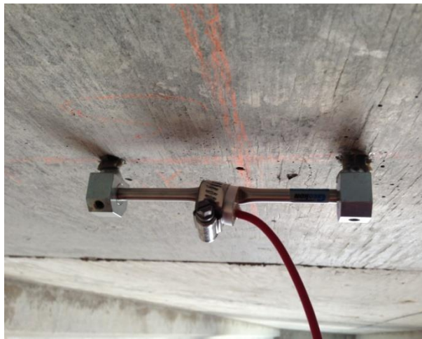
Figure 16. Vibrating wire strain gauge at the bottom of the deck
