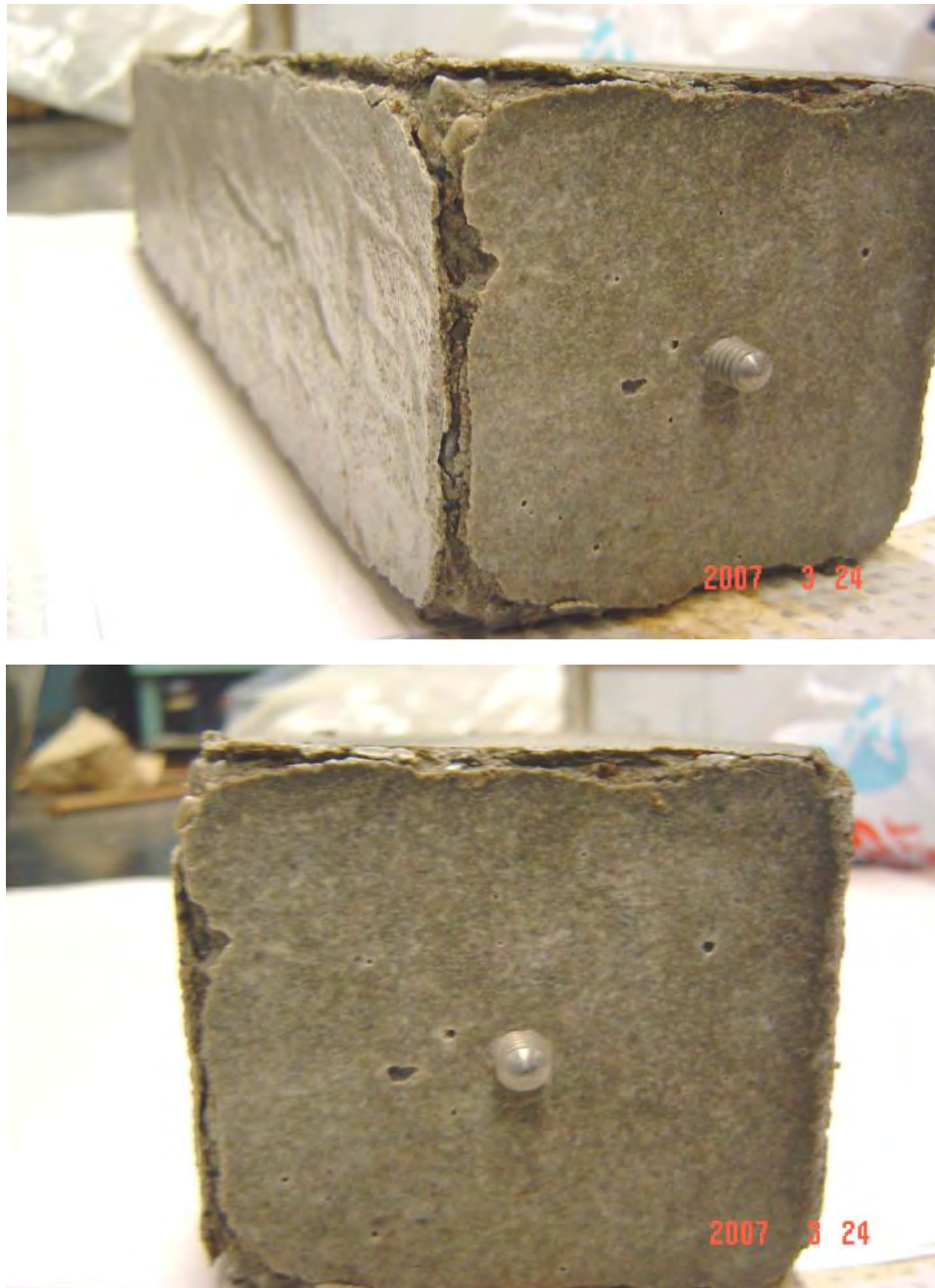
Figure A3.229. Photographs of concrete prisms subjected to 133 freezing and thawing cycles in 15% \text{CaCl}_2 solution.
