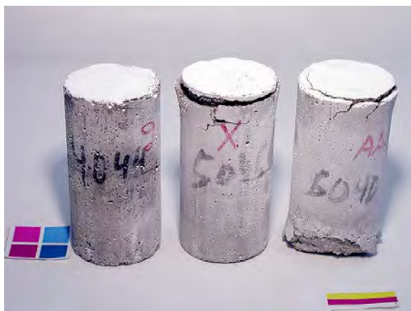
Figure A3.75. Cylinders exposed to \text{CaCl}_2 solution after 56 days of constant low temperature test. From left to right: 0.40, 0.50, and 0.60 w/c mortar cylinders. Solution strength was 17% \text{CaCl}_2 .
