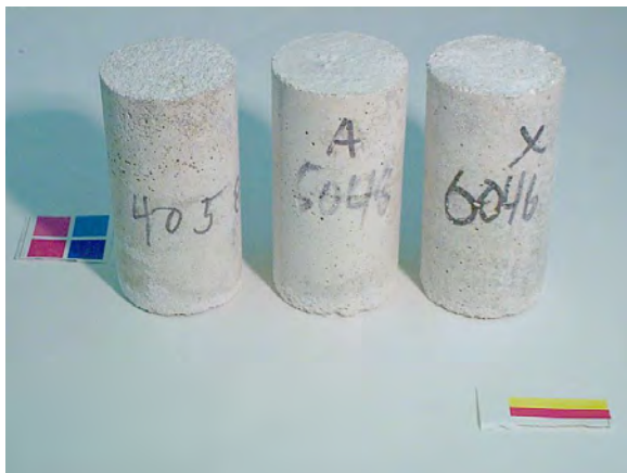
Figure A3.59. Cylinders exposed to NaCl solution after 84 days of constant high temperature test. From left to right: 0.40, 0.50, and 0.60 w/c mortar cylinders.
