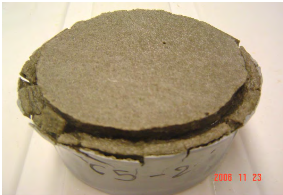
Figure A3.91. Deteriorated disc sample exposed to 28% \text{CaCl}_2 after 150 days of exposure.
