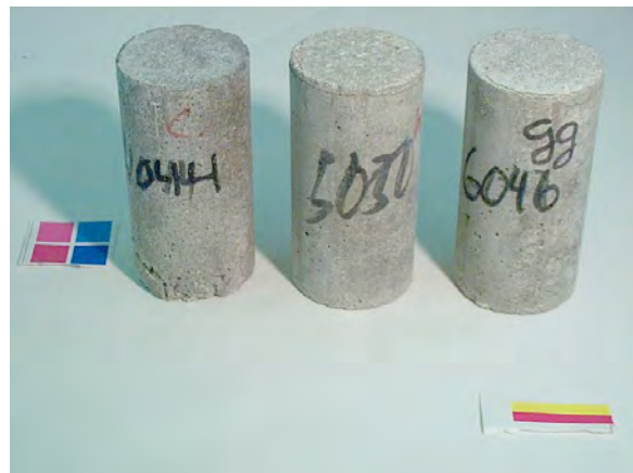
Figure A3.60. Cylinders exposed to MgCl 2 solution after 84 days of constant high temperature test. From left to right: 0.40, 0.50, and 0.60 w/c mortar cylinders.
