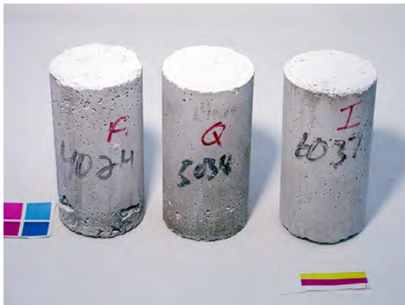
Figure A3.73. Cylinders exposed to \text{CaCl}_2 solution after 56 days of constant low temperature test. From left to right: 0.40, 0.50, and 0.60 w/c mortar cylinders. Solution strength was 10% \text{CaCl}_2 .
