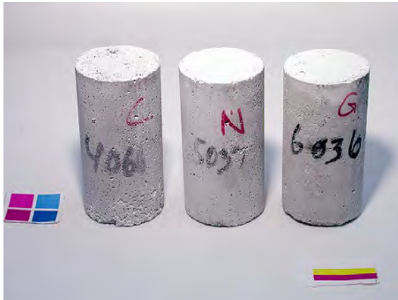
Figure A3.71. Cylinders exposed to \text{CaCl}_2 solution after 56 days of constant low temperature test. From left to right: 0.40, 0.50, and 0.60 w/c mortar cylinders. Solution strength was 3% \text{CaCl}_2 .
