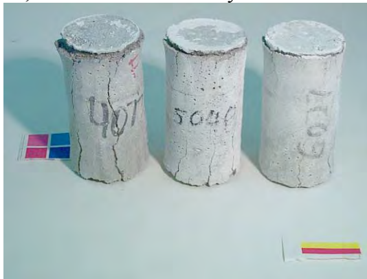
Figure A3.21. Cylinders exposed to CaCl_2 solution after 84 days of constant low temperature test. From left to right: 0.40, 0.50, and 0.60 w/c mortar cylinders.
