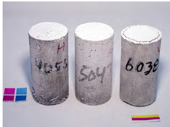
Figure A3.74. Cylinders exposed to \text{CaCl}_2 solution after 56 days of constant low temperature test. From left to right: 0.40, 0.50, and 0.60 w/c mortar cylinders. Solution strength was 14% \text{CaCl}_2 .
