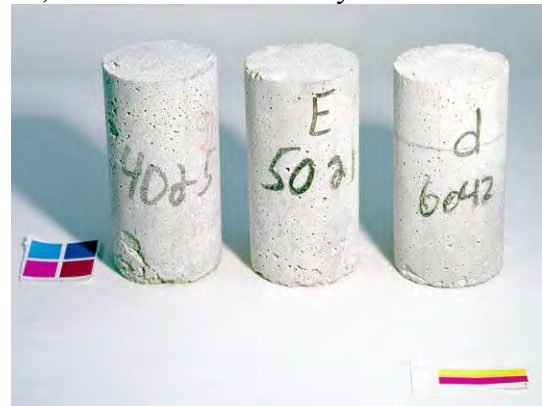
Figure A3.22. Cylinders exposed to CMA solution after 84 days of constant low temperature test. From left to right: 0.40, 0.50, and 0.60 w/c mortar cylinders.
