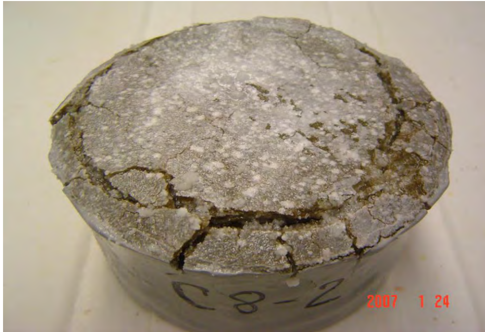
Figure A3.90. Deteriorated disc sample exposed to 20% \text{MgCl}_2 after 150 days of exposure.
