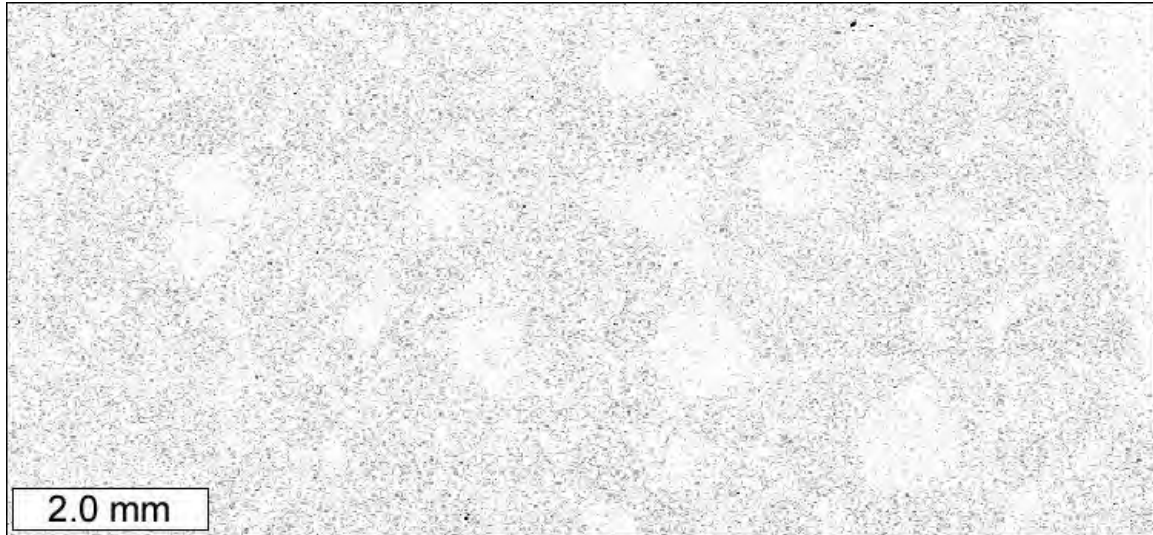
Figure A3.13. Sodium K\alpha X-ray map from control cylinder. Darker areas correspond to higher K\alpha X-ray counts.
