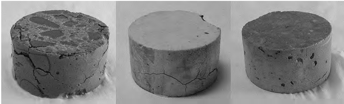
Figure A3.128. Photographs of 4 inch [100 mm] diameter 0.45 w/c ordinary portland cement (OPC) concrete specimens after 500 days in high concentration brines. From left to right: CaCl 2 , MgCl 2 , and MBAP brines.
