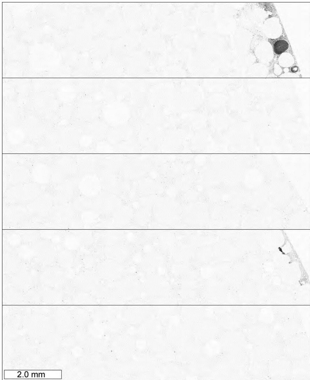
Figure A3.30. Elemental map for magnesium collected from thin sections prepared from mortar cylinders immersed in the following solutions, from top to bottom: magnesium chloride, calcium chloride, sodium chloride, calcium magnesium acetate, and limewater. Darker areas indicate a higher concentration.
