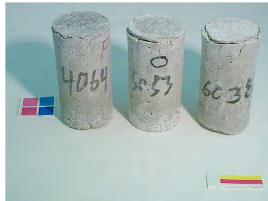
Figure A3.20. Cylinders exposed to MgCl_2 solution after 84 days of constant low temperature test. From left to right: 0.40, 0.50, and 0.60 w/c mortar cylinders.
