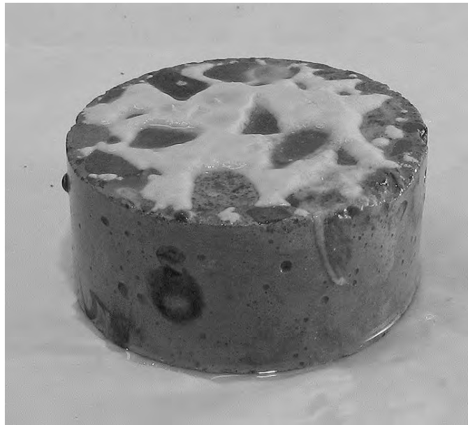
Figure A3.130. White precipitate on exterior of 4 inch [100 mm] diameter concrete specimen after 500 days immersion in low-concentration CMA solution.
