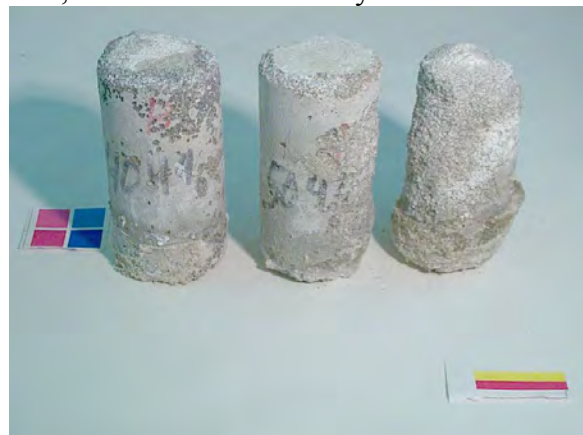
Figure A3.62. Cylinders exposed to CMA solution after 28 days of constant high temperature test. From left to right: 0.40, 0.50, and 0.60 w/c mortar cylinders.
