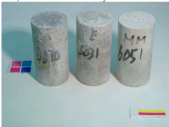
Figure A3.61. Cylinders exposed to CaCl 2 solution after 84 days of constant high temperature test. From left to right: 0.40, 0.50, and 0.60 w/c mortar cylinders
