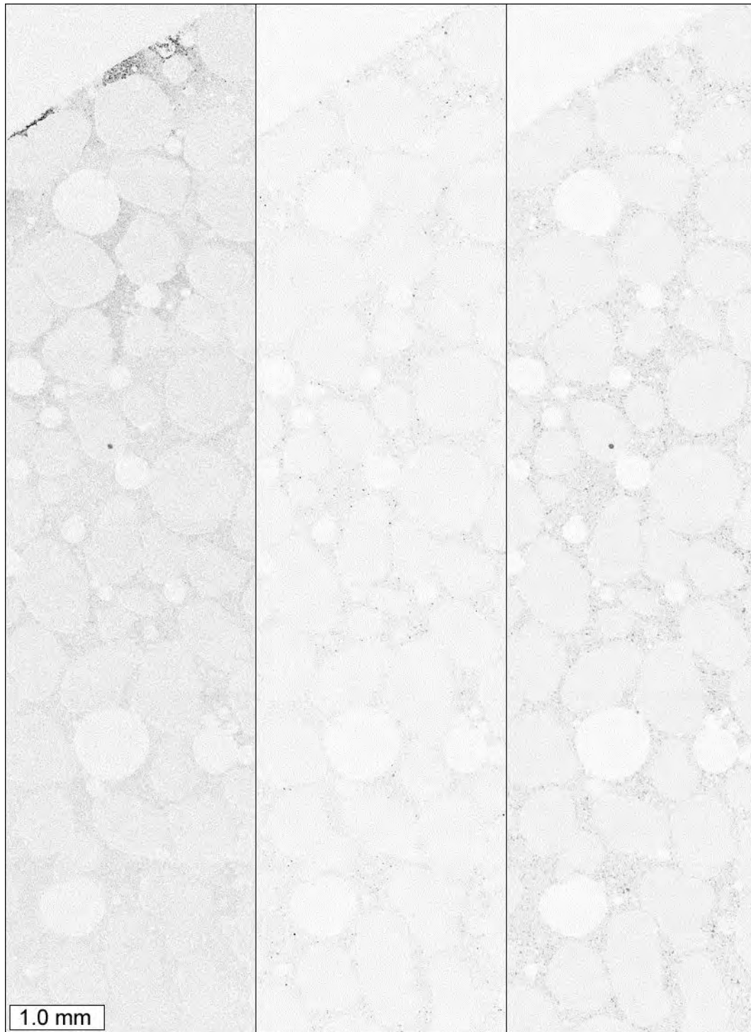
Figure A3.46. Elemental maps, from left to right: sodium, magnesium, and aluminum. The elemental maps were collected from a thin section prepared from a cylinder immersed in sodium chloride solution. Darker areas indicate a higher concentration.
