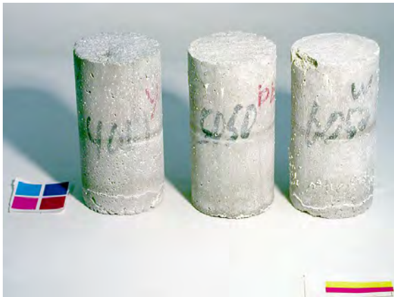
Figure A3.5. Cylinders exposed to CMA solution after 84 days of cyclic temperature test. From left to right: 0.40, 0.50, and 0.60 w/c mortar cylinders.
