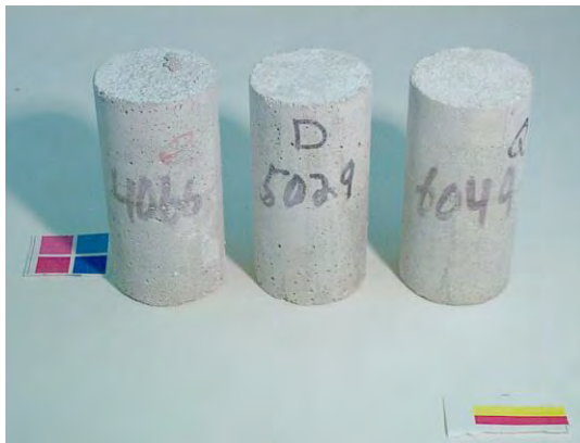
Figure A3.19. Cylinders exposed to NaCl solution after 84 days of constant low temperature test. From left to right: 0.40, 0.50, and 0.60 w/c mortar cylinders.
