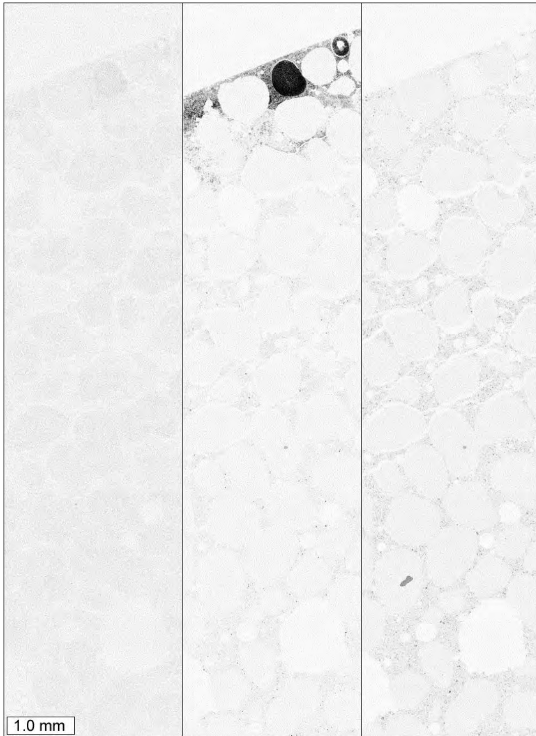
Figure A3.36. Elemental maps, from left to right: sodium, magnesium, and aluminum. The elemental maps were collected from a thin section prepared from a cylinder immersed in magnesium chloride solution. Darker areas indicate a higher concentration.
