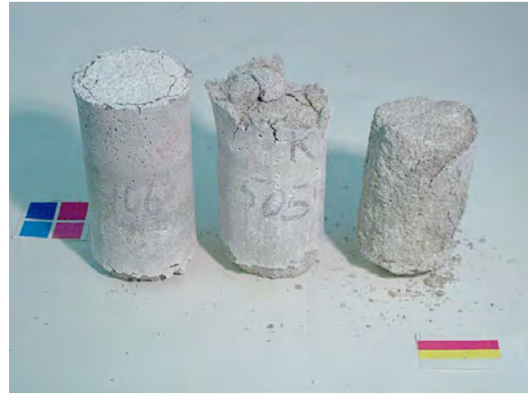
Figure A3.4. Cylinders exposed to \text{CaCl}_2 solution after 84 days of cyclic temperature test. From left to right: 0.40, 0.50, and 0.60 w/c mortar cylinders.
