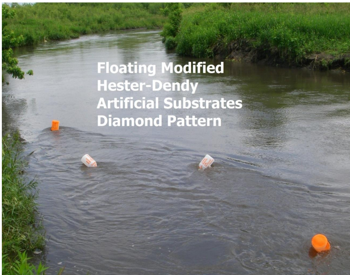
Photographs showing the diamond deployment pattern for standard and floating modified Hester-Dendy artificial substrates.
