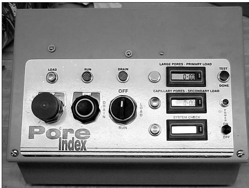
Figure 2. Control panel with (from right to left) Stop button, Start button, Mode Switch, indicator lights, digital timers, and power switch.
