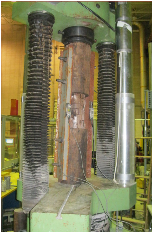
Timber sistered with steel was one of the two solutions that was laboratory tested
