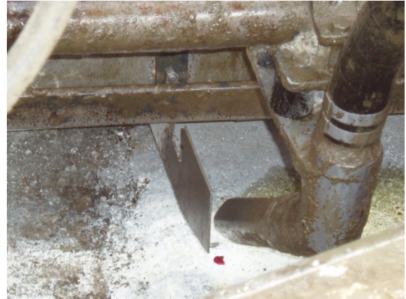
Figure 14. Longitudinal Joint “Knife” Installed on Slipform Paver
