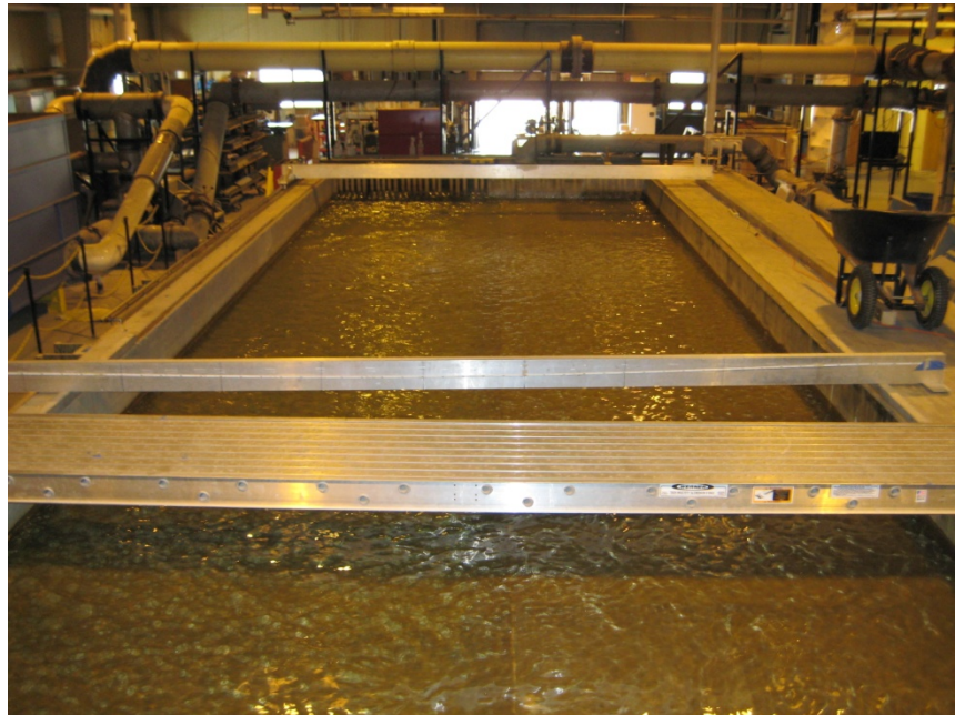
Figure 9. View looking upstream of the 21.3 m long, 4.0 m wide recirculating flume.
