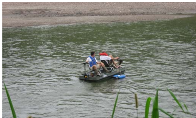
Figure 16. Detection of the particles in the Raccoon River via the floatable antenna towed by the boat.
