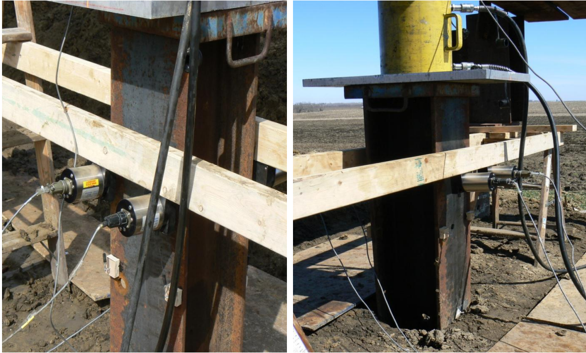
Figure 4.20. Pile top vertical displacement transducers instrumentation
