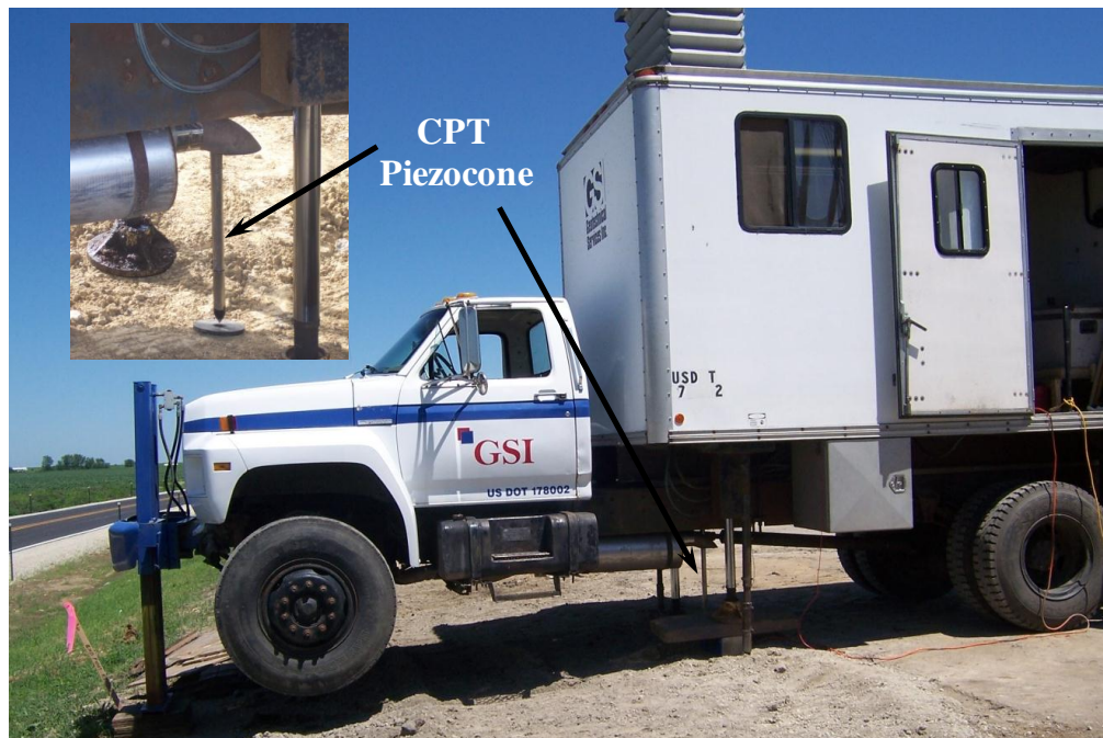
Figure 3.3. Typical Cone Penetration Test (CPT)
