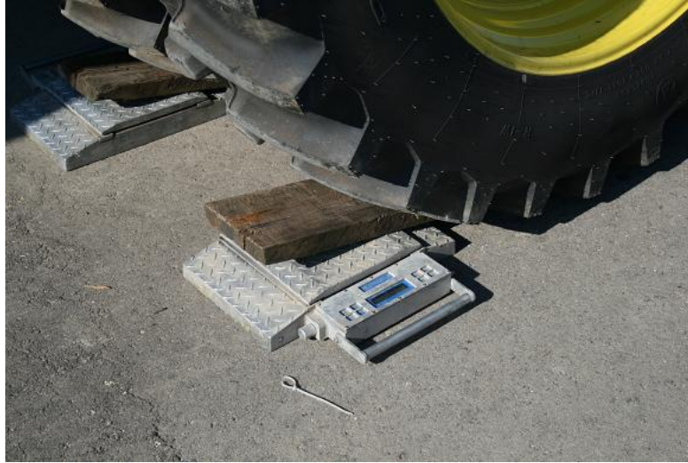
Figure 3.16. Weighing vehicles using portable scales
