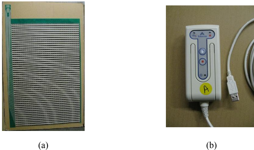
Figure 3.19. Tekscan hardware components (a) 5400N sensor mats (b) Evolution Handle
