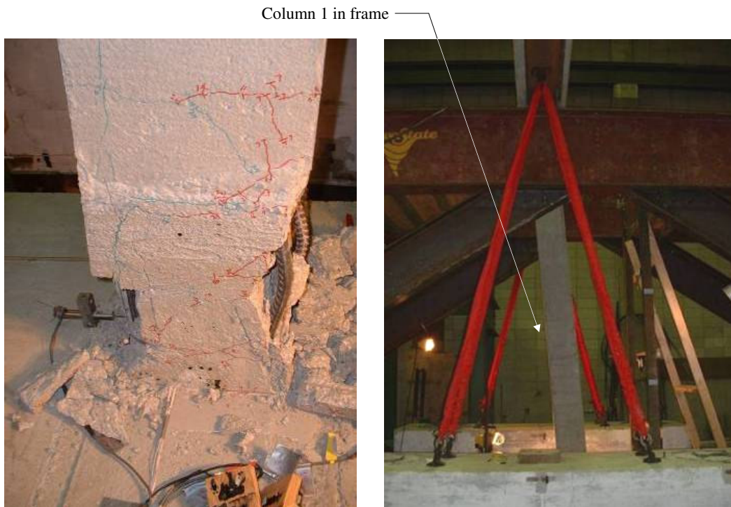
Figure 83. Photographs of Column 1 - Cycle 27 damage and deformation.
