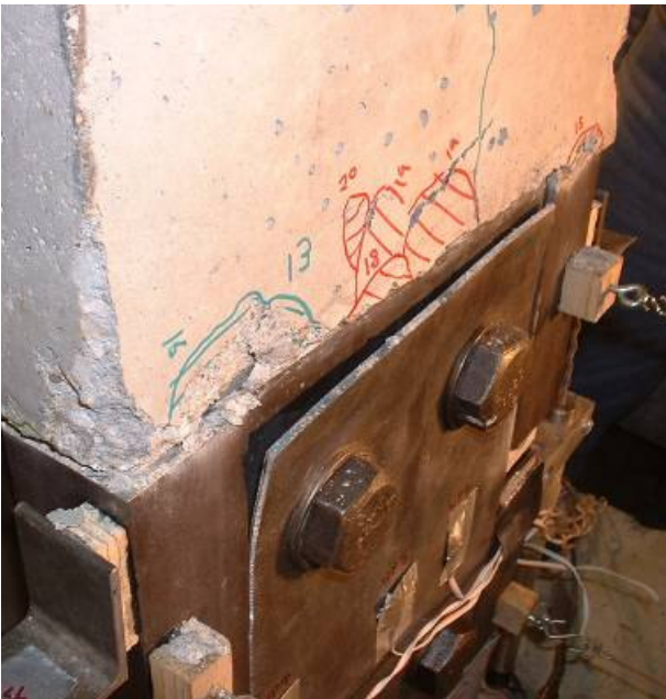
c.) West bolt bearing causing plate curling
