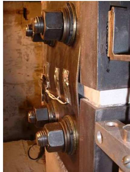
b.) Initial buckling of east plate
