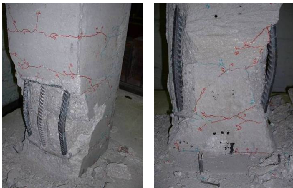
Figure 83. Photographs of Column 1 - Cycle 27 damage and deformation.
