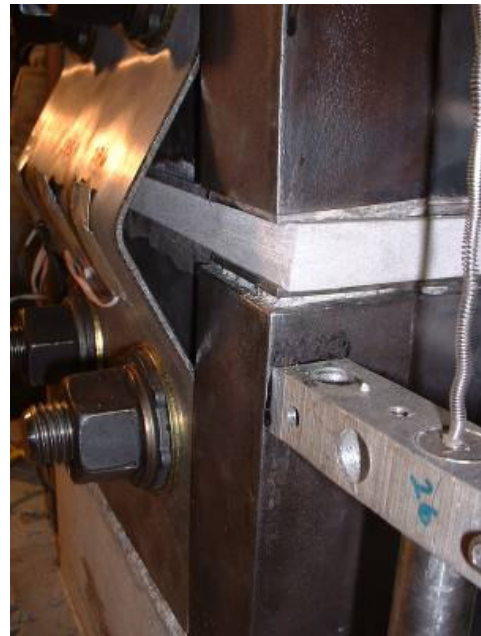
d.) East fuse plate buckling
