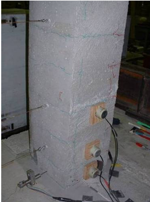
a.) Southwest corner view of progressive cracking
