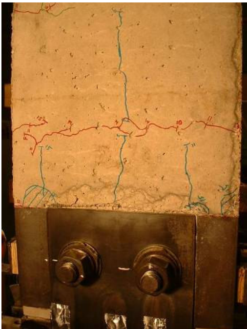
c.) East face cracking above top collar
