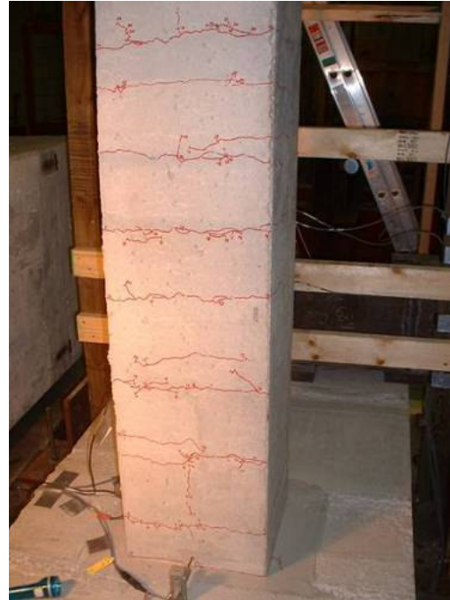
b.) Progressive cracking on the east face
