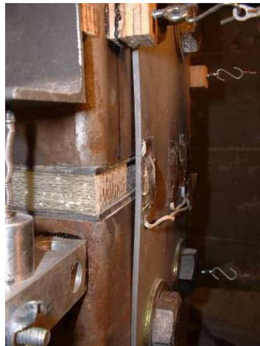
a.) East face of upper segment crack distribution b.) West fuse plate initial buckling
