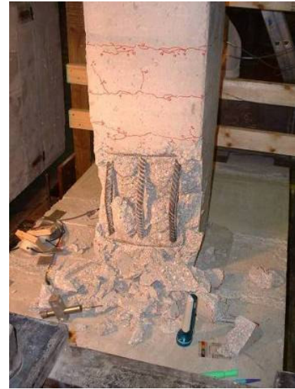
b.) East face reinforcement exposed
