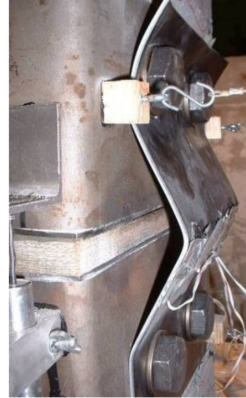
b.) West fuse plate buckling
