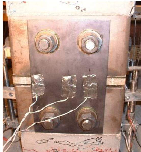
b.) East joint opening during push half-cycle
