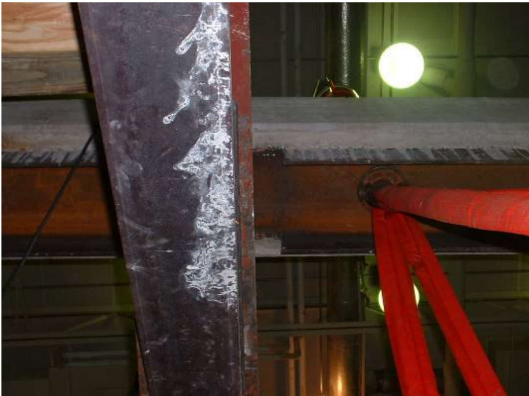
c.) Load beam impinging on load frame
