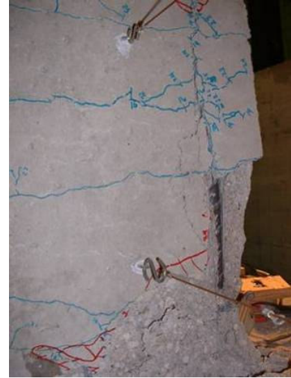
b.) Visible southwest corner reinforcement
