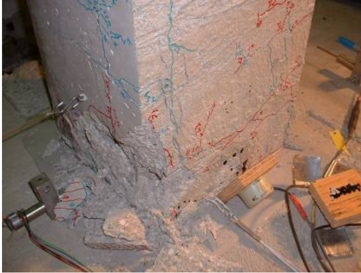
a.) Severe spalling of southwest corner
