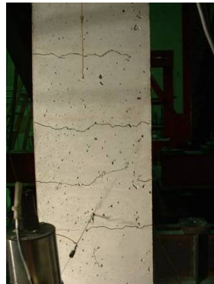
b.) Upper segment crack progression
