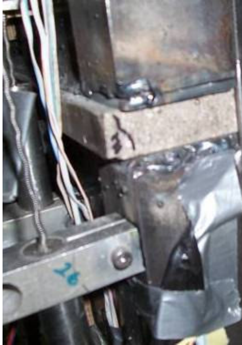
a.) Damage to bearing plate in southeast corner
