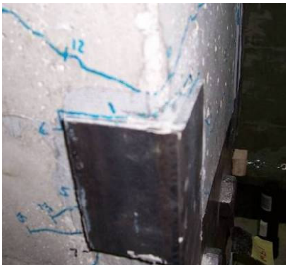
a.) Cracks forming around southeast retrofit angle
