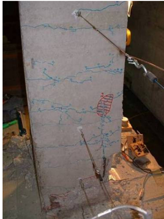
d.) West face damage
