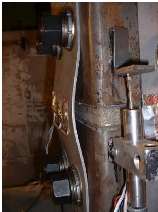
b.) East fuse plate buckling
