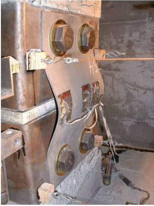
a.) West fuse plate buckling
