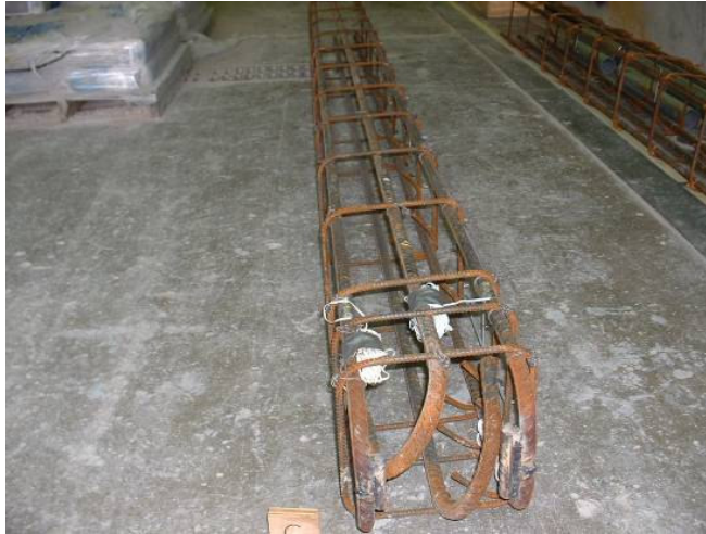
Figure 48. Photograph of Column 4, 12 ft. segment reinforcement.
