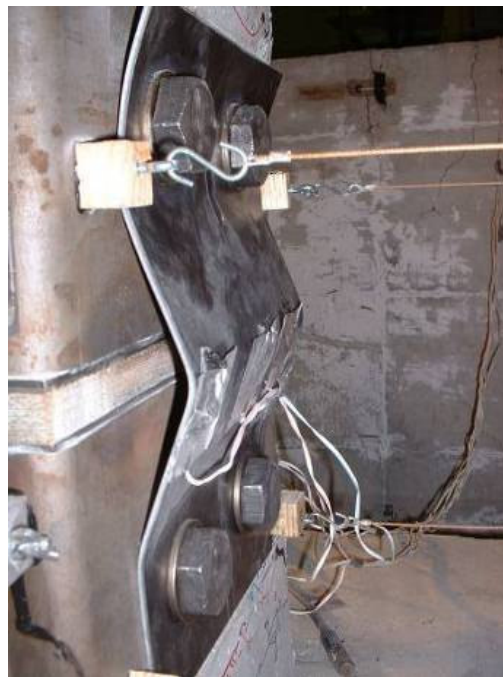
c.) West fuse plate buckling
