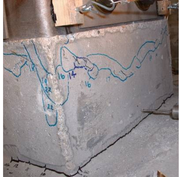
b.) Lower segment west face compression damage
