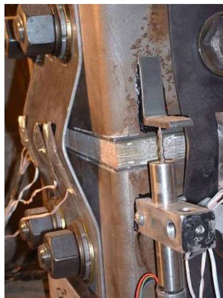
d.) Northeast corner fuse plate buckling
