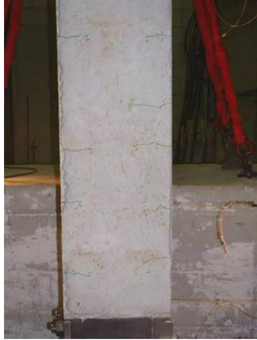
b.) North face crack progression
