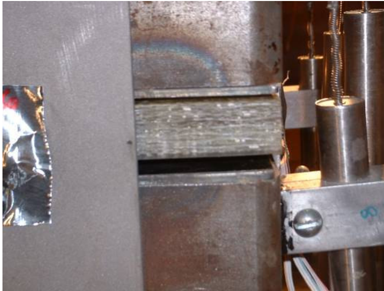
Figure 154. Photograph of Column 6 – Cycle 26b, east joint opening.
