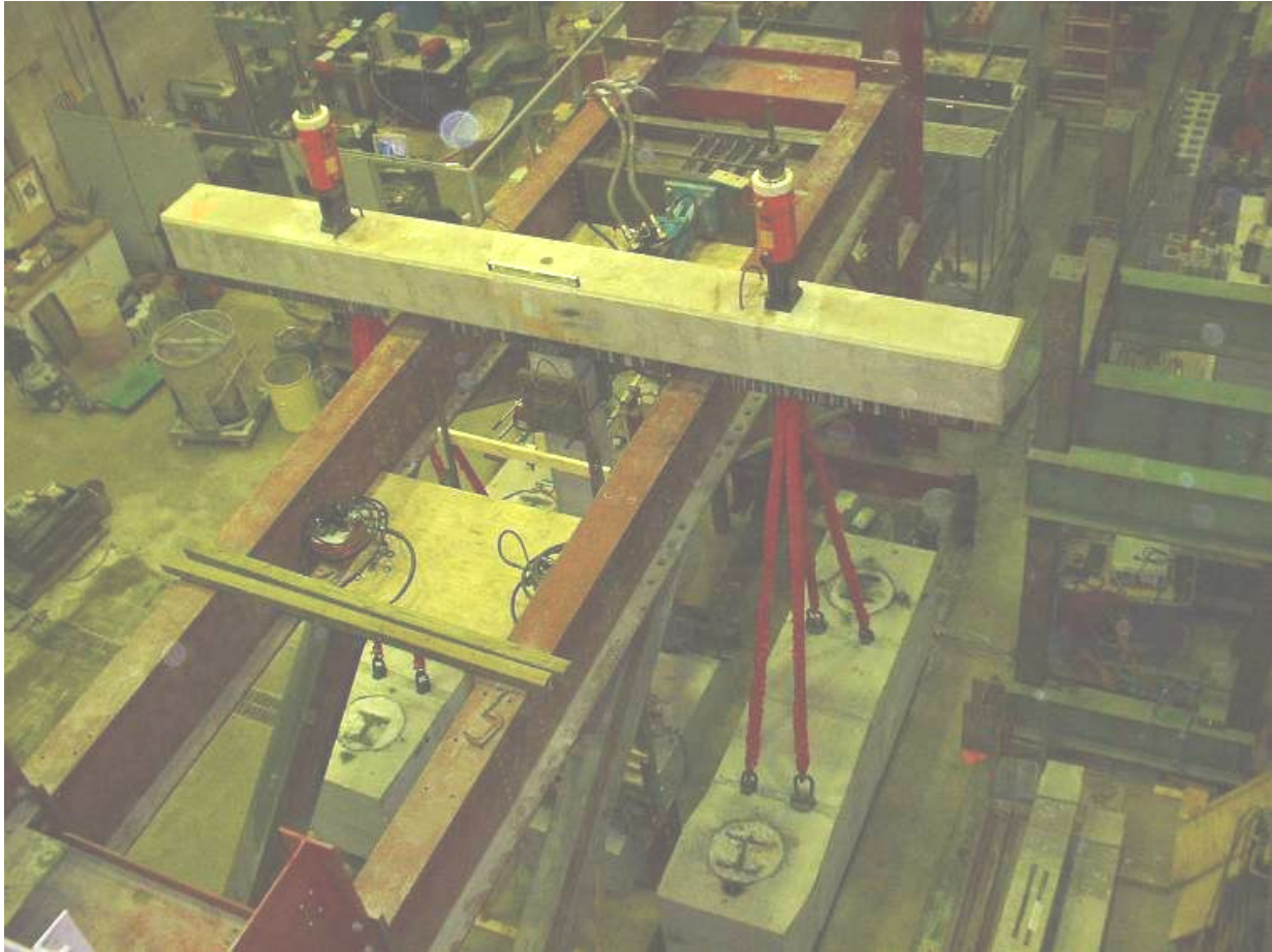
Figure 8. Photograph of load beam from above.
