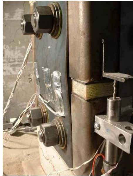
b.) East plate initial buckling
