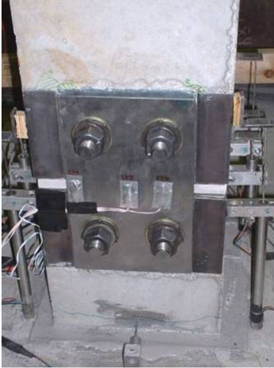
a.) East replacement fuse plate
