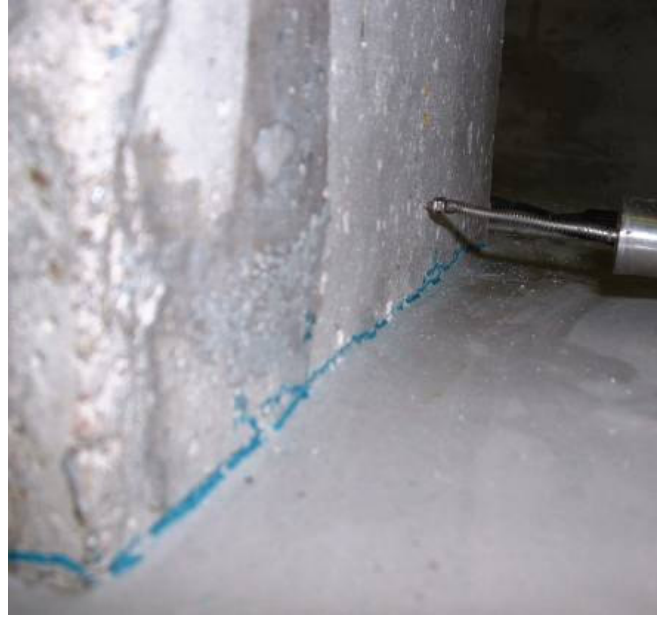
b.) West face initial cracking
