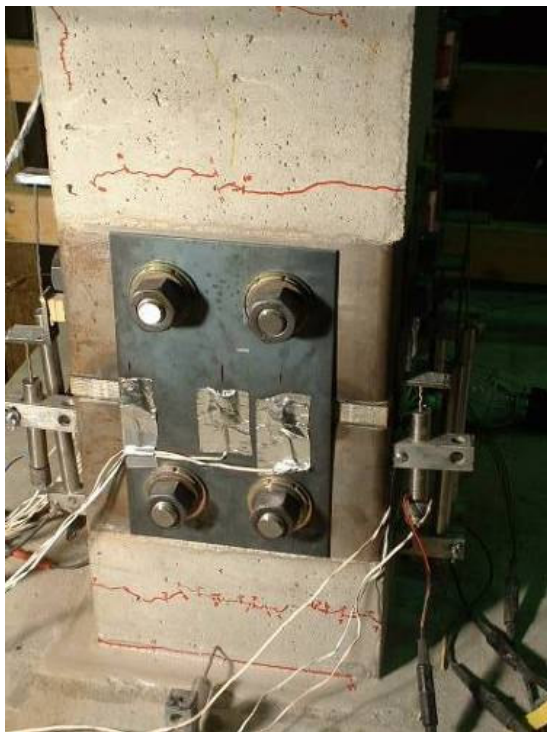
a.) Cracking around column joint
