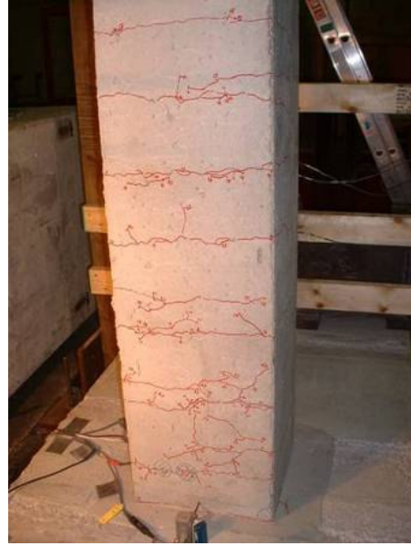
b.) East face crack progression
