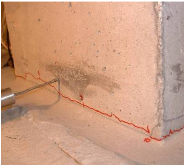
a.) East face initial cracking
