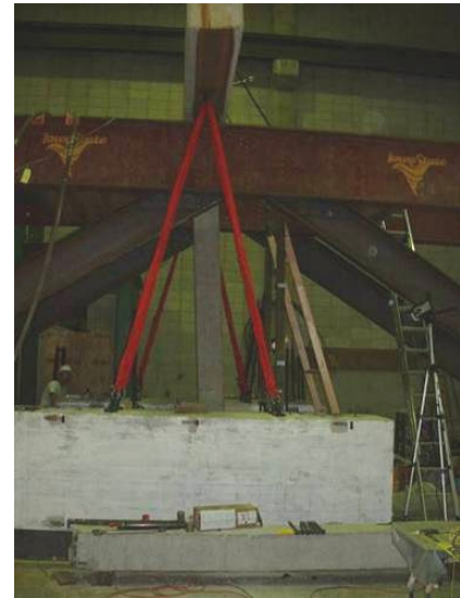
d.) Column tilt during negative half-cycle
