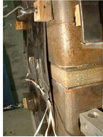
b.) West fuse plate initial buckling
