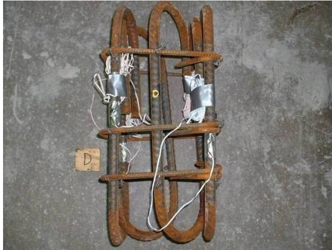
Figure 42. Photograph of Column 3, 2 ft. segment reinforcement.
