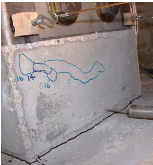
a.) West face initial compression damage
