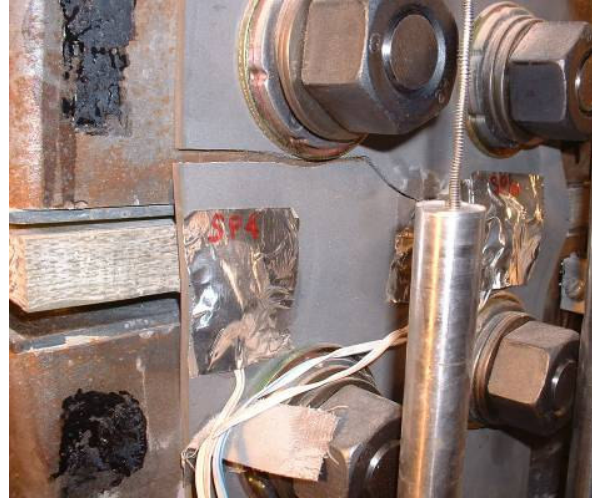
b.) Fuse plate crack at -9.0 in. displacement
