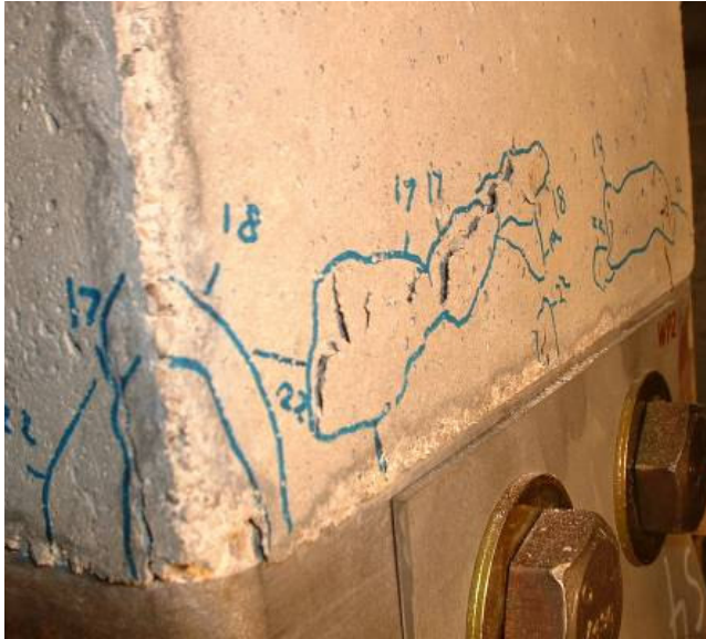
a.) Upper segment west face compression damage
