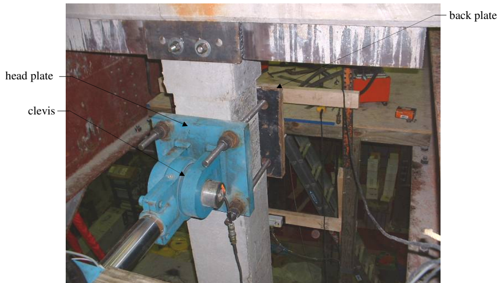
Figure 10. Photograph of actuator connection to column.
