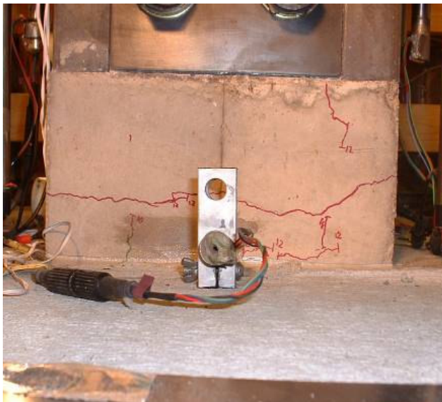
a.) East base cracking
