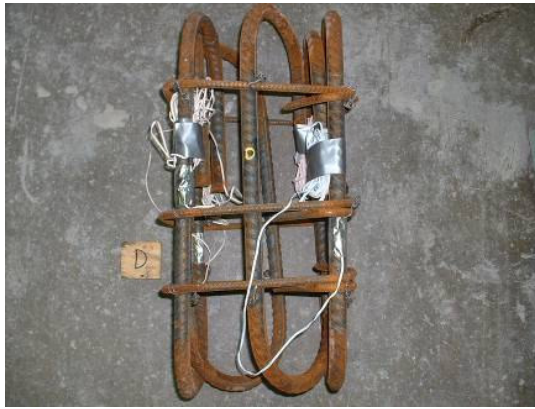
a.) Columns 2-4, 2 ft. segment reinforcement
