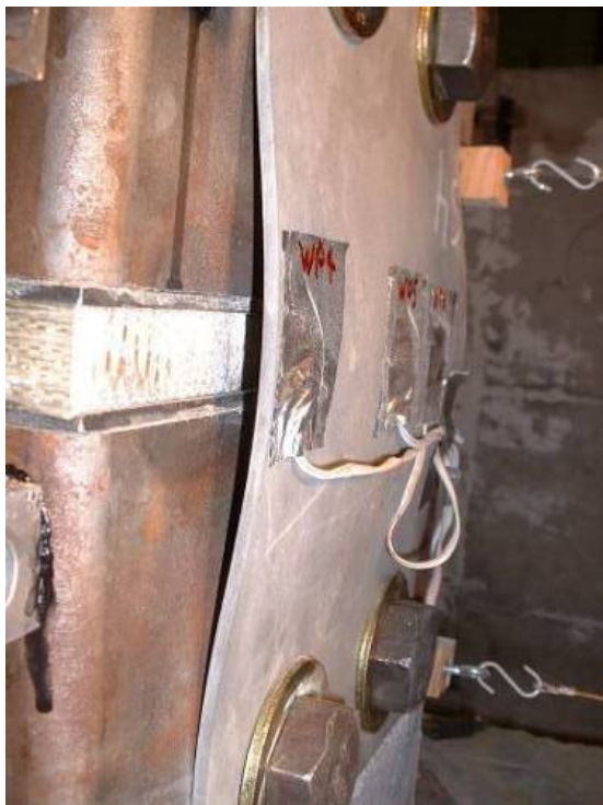
a.) West fuse plate buckling
