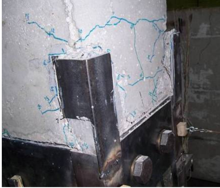
b.) Upper segment damage and retrofit failure
