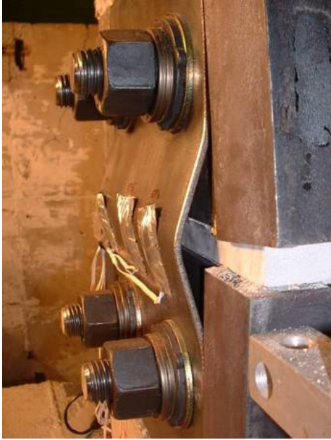
a.) East plate buckling during last cycle
