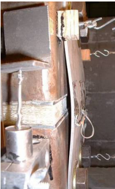
a.) West fuse plate buckling
