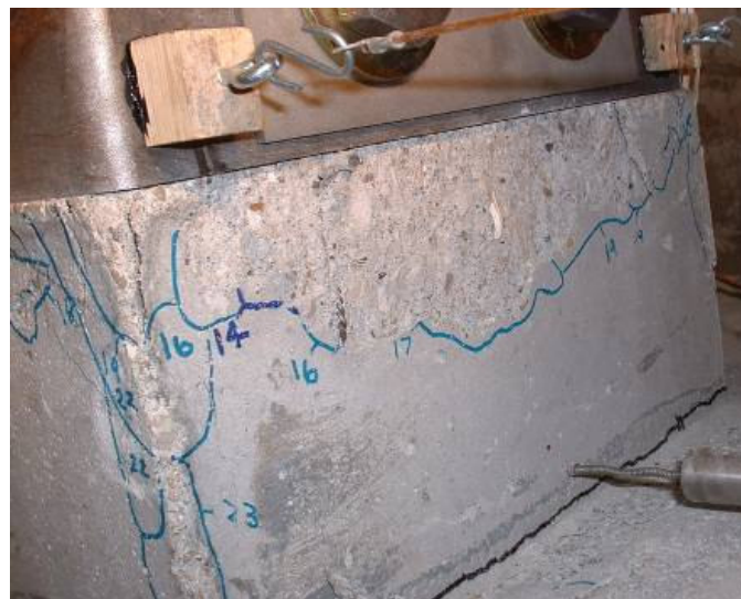
b.) Lower segment west face spalling
