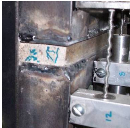
b.) Northeast corner bearing plate compression damage
