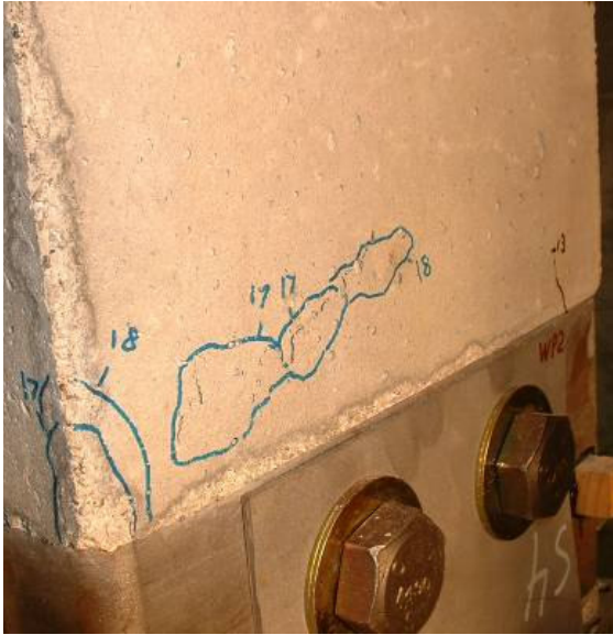
a.) Upper west column segment compression damage
