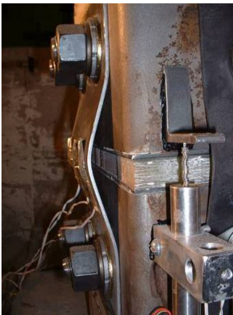
a.) East fuse plate buckling
