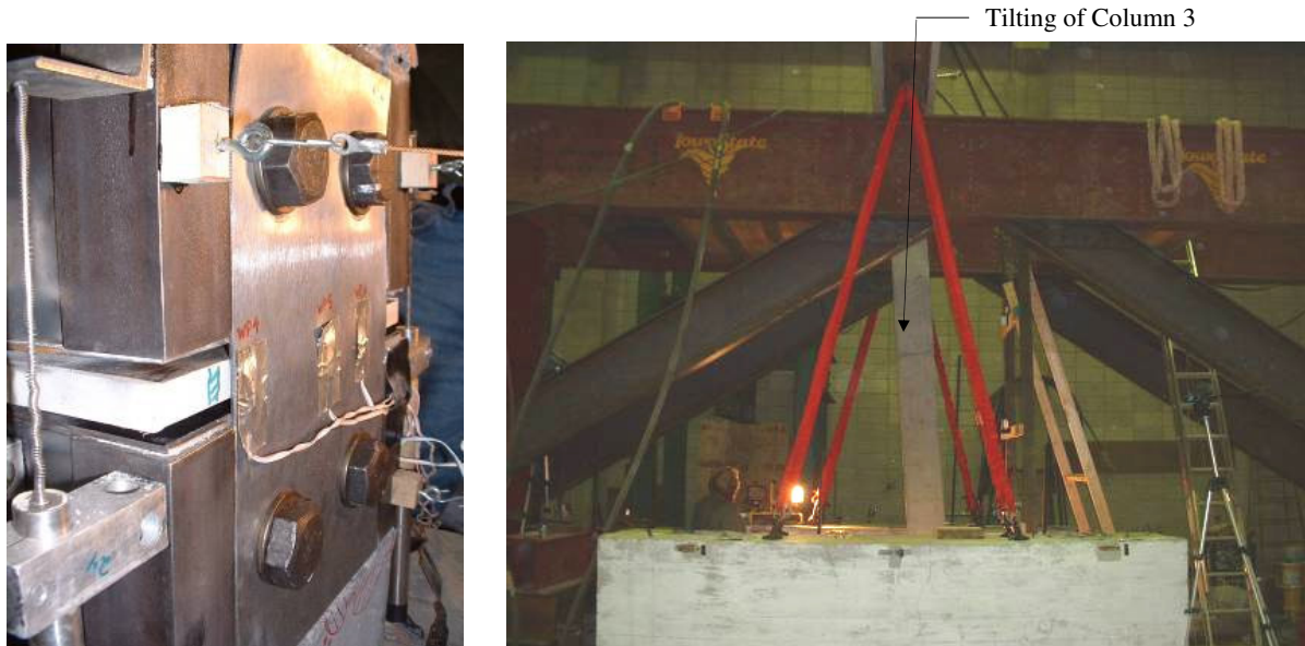
a.) Northeast corner joint opening
