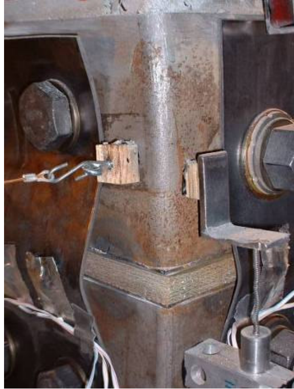
b.) Southwest corner fuse plate buckling
