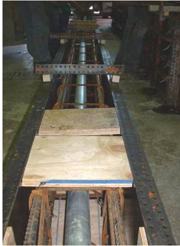
Figure 45. Photograph of Column 3 reinforcement and inserts.
