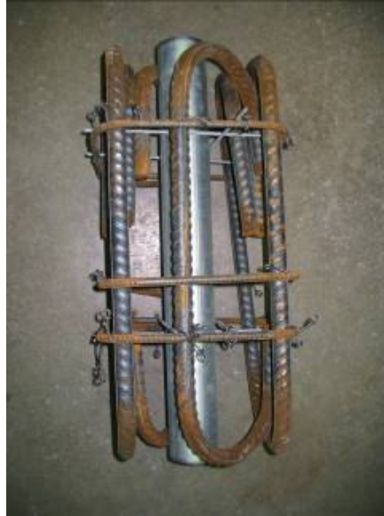
Figure 38. Photograph of reinforcement of Column 2 (2 ft. column segment).
