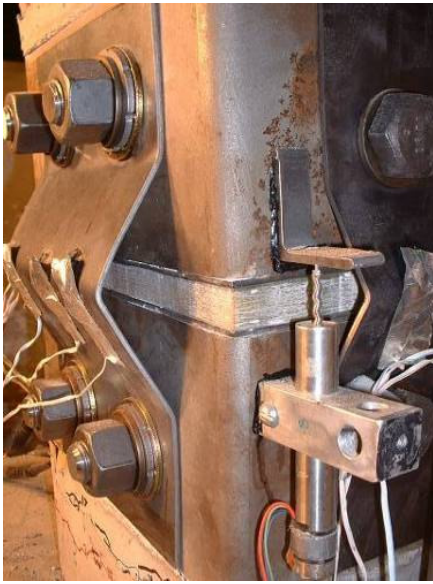
a.) East fuse plate buckling
