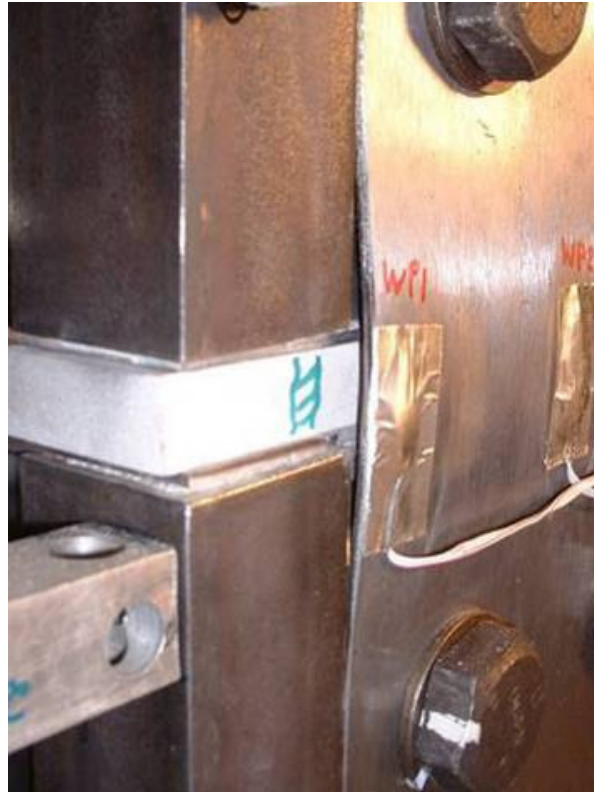
c.) Initial buckling of fuse plate and compression damage in bearing plate
