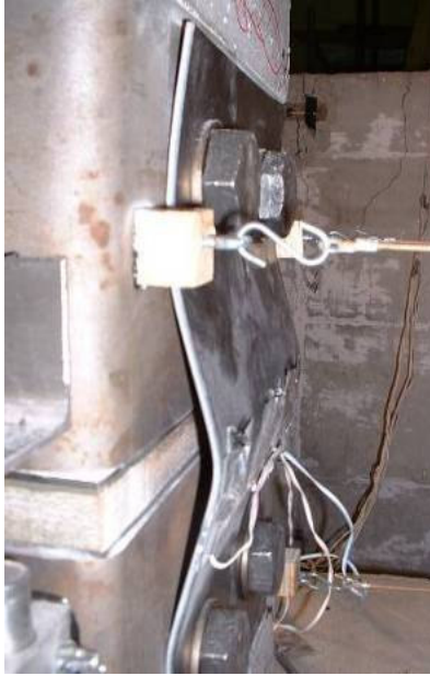
a.) West fuse plate buckling
