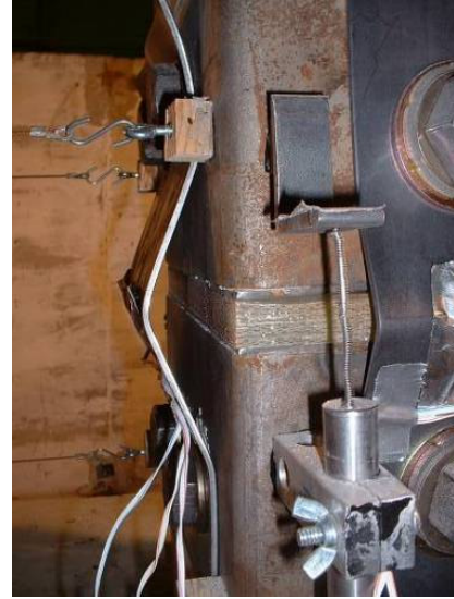
b.) West fuse plate buckling
