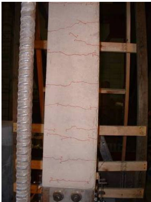
a.) East face of upper segment crack distribution b.) West fuse plate initial buckling
