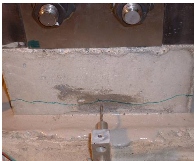
b.) East base initial cracking
