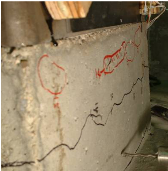
a.) West face compression damage and cracking at base
