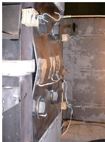
d.) Buckling of replaced west plate
