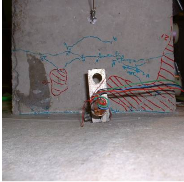
b.) Localization of compression damage on southwest corner
