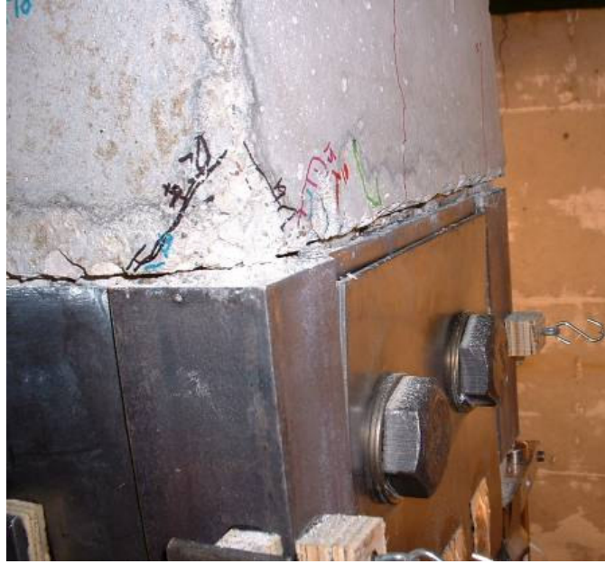
b.) West collar/column interface final crack width
