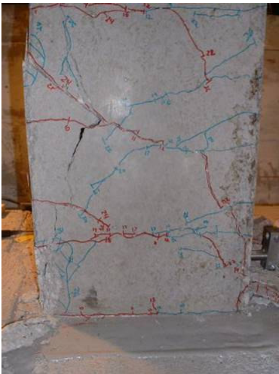
c.) North face cracking/spalling
