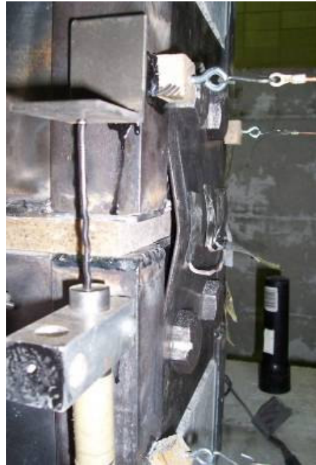
b.) West fuse plate buckling
