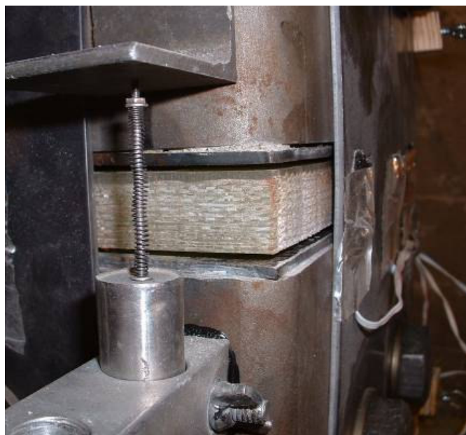
b.) West joint opening during pull half-cycle
