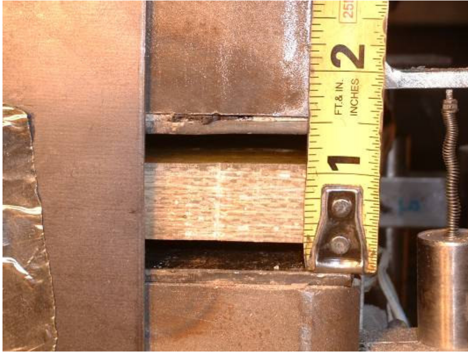
a.) East joint opening during push half-cycle
