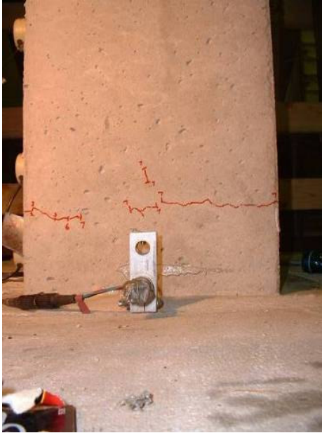
a.) East face initial cracking
