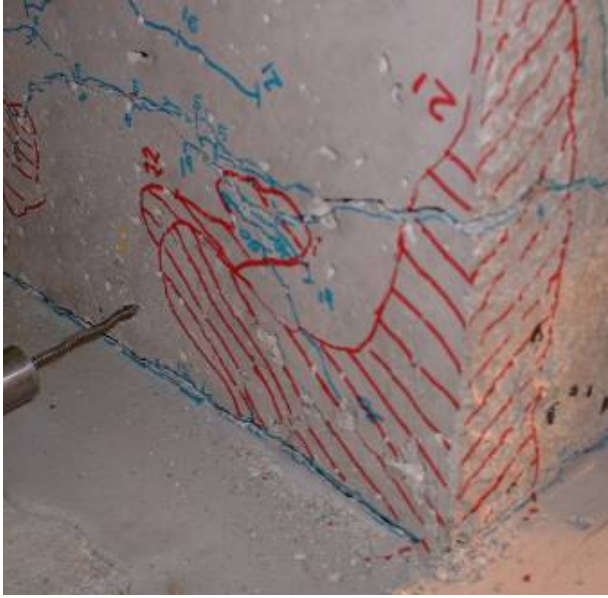
a.) Southwest corner compression damage
