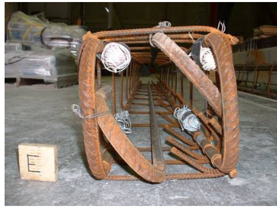
b.) Columns 2-4, 12 ft. segment reinforcement
