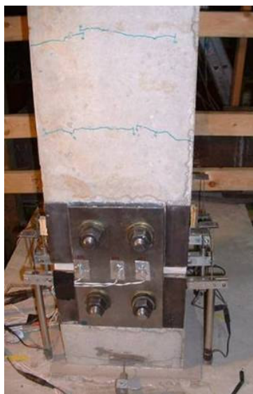
a.) East face crack progression
