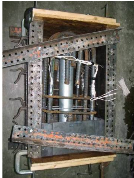
Figure 39. Photograph of Column 2 reinforcement in forms.
