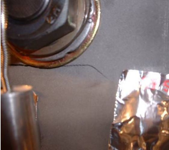
a.) Initial fracture of south fuse plate at -5.22 in. displacement
