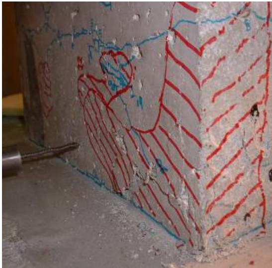
a.) Southwest corner compression damage
