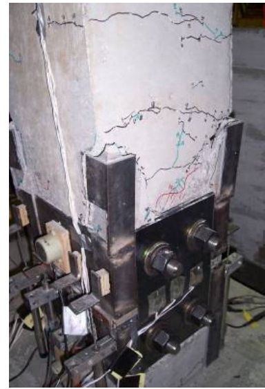
b.) East face column damage
