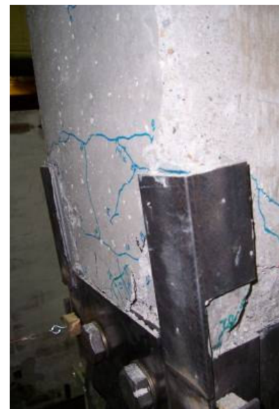
b.) Upper column segment damage
