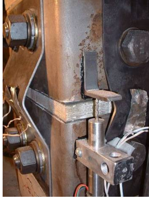
b.) East fuse plate buckling
