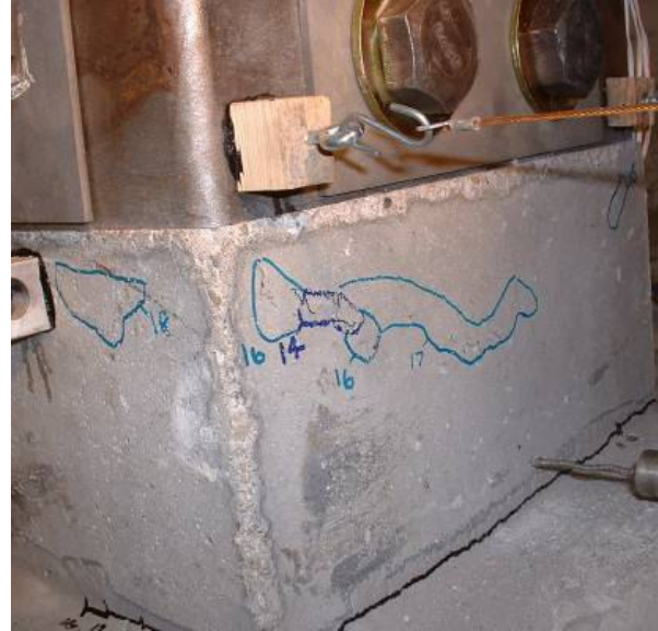
b.) Northwest corner compression damage
