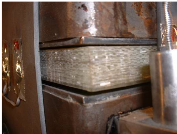
Figure 150. Photographs of Column 6 – Cycle 21b, joint opening.
