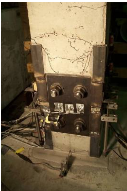
a.) East face crack progression
