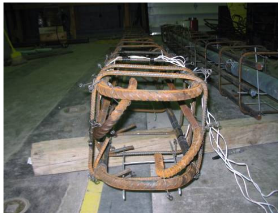
Figure 15. Base end of control column reinforcement cage.
