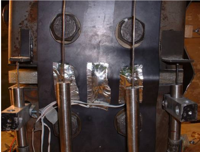
a.) North fuse plate differential buckling
