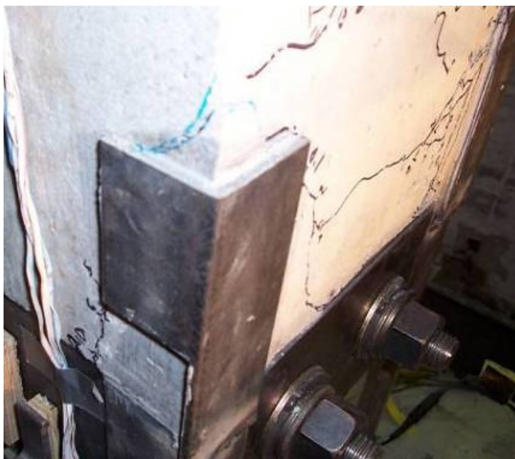
b.) Incipient cracking at southeast retrofit angle
