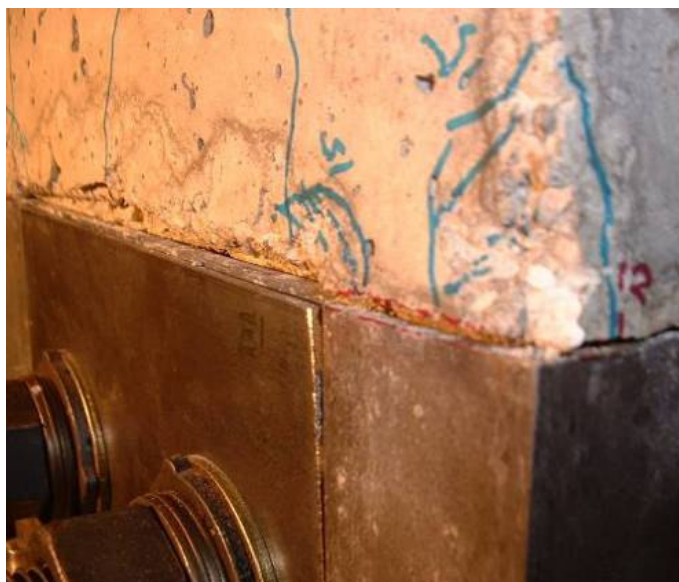
b.) Northeast corner collar/column interface
