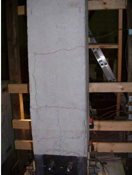
a.) East face crack progression
