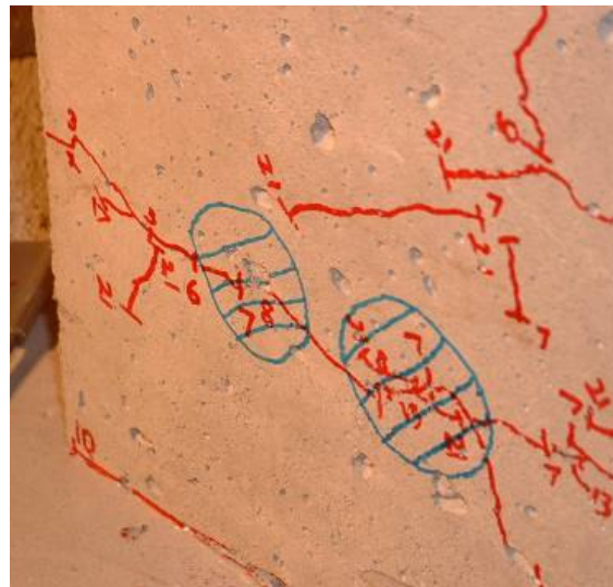
b.) East face initial compression damage
