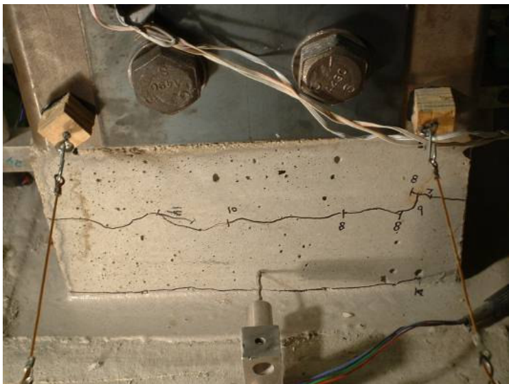
a.) Cracking at the base of the west face
