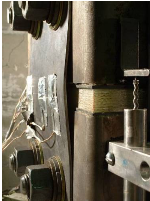
b.) East plate buckling in compression
