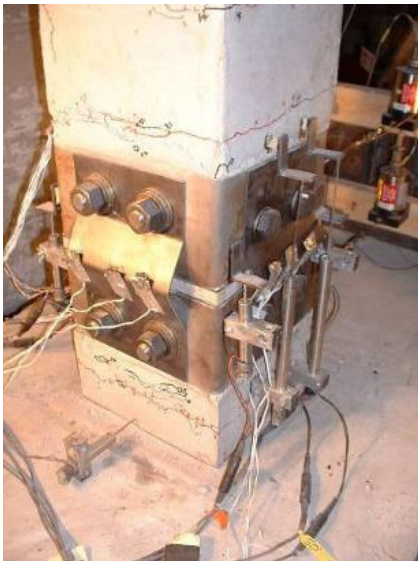
a.) Residual fuse plate buckling
