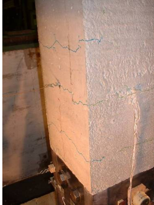
b.) Southwest corner crack progression
