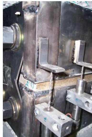
d.) Northeast corner fuse plate buckling
