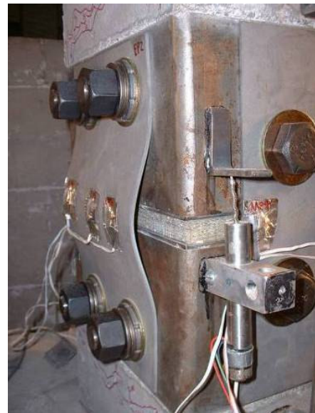
d.) West fuse plate buckling
