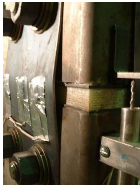
b.) East fuse plate buckling
