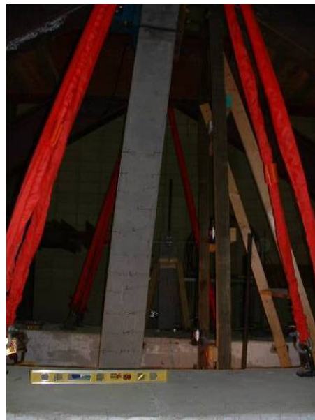
d.) Column deformation during push half-cycle
