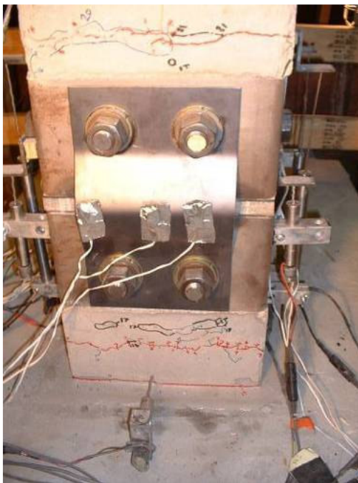
b.) East fuse plate buckling and segment damage
