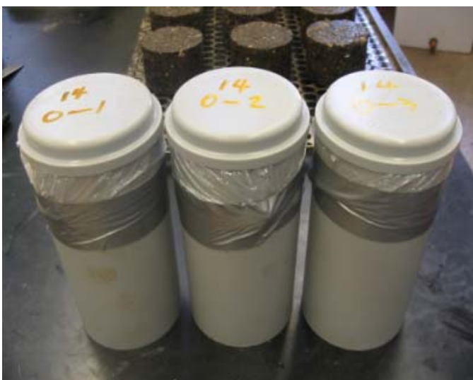
Figure 4-1. Pictures of three curing conditions for CIR specimens
