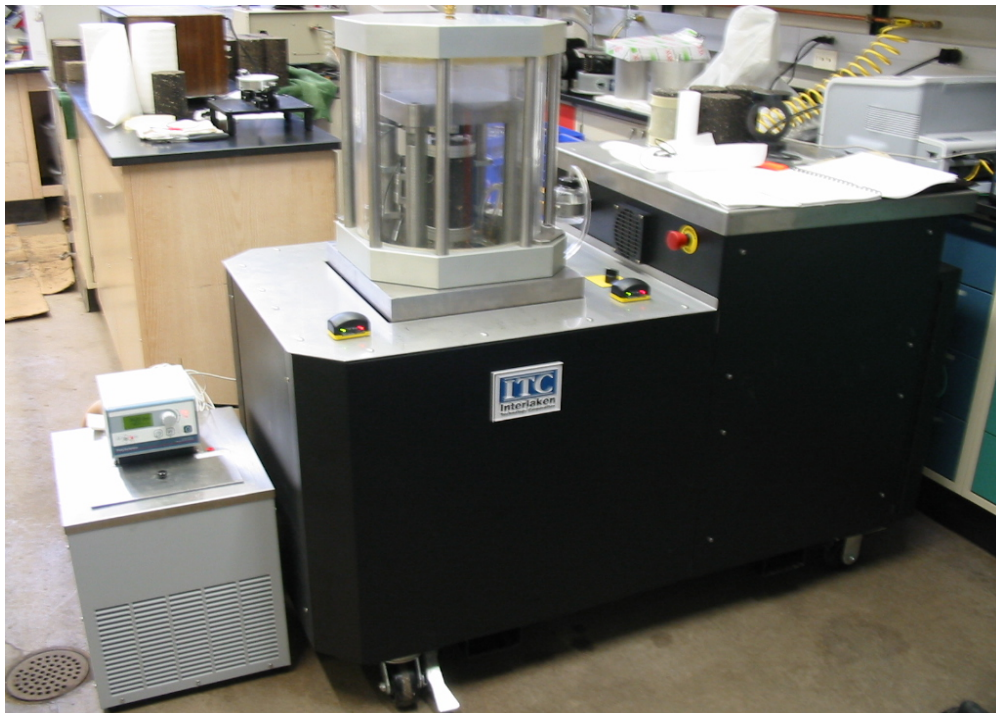
Figure 8-1. Simple performance testing equipment at the University of Iowa
