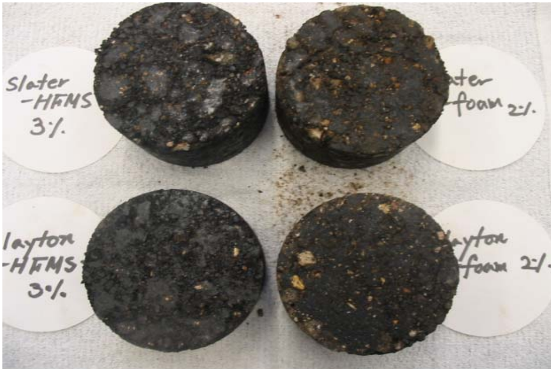
Figure 6-2. Visual observation of gyratory compacted CIR-foam and CIR-emulsion specimens
