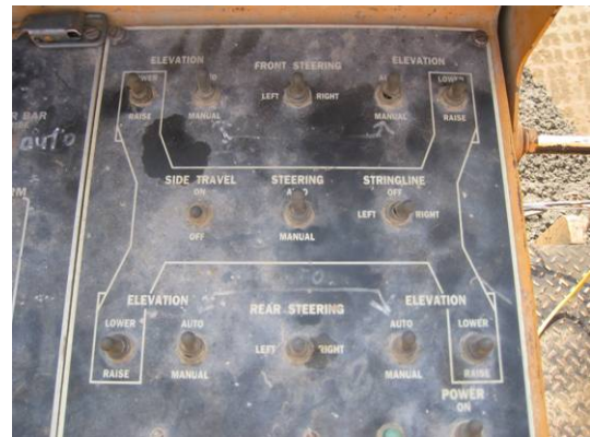
Figure 8. Current Control Panel on CMI Paving Machine
