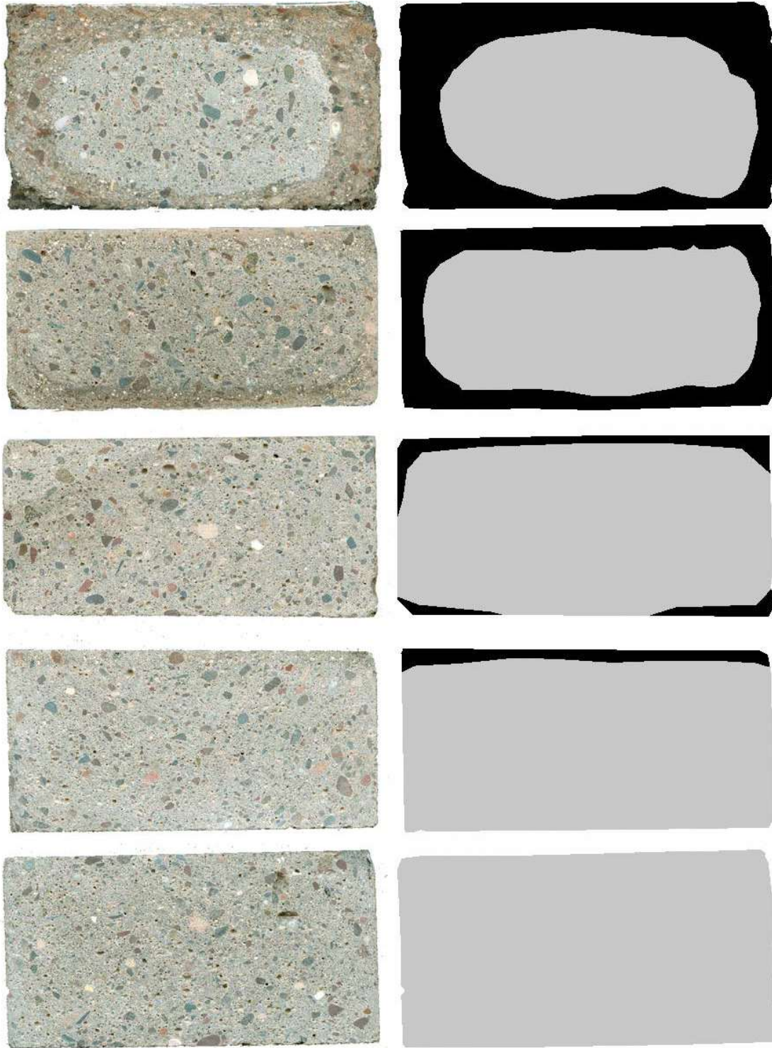
Figure 38. Visible alteration on saw-cut plane through 0.45 w/c mortar specimens, from top to bottom: CaCl 2 , MgCl 2 , MBAP, NaCl & CMA high-concentration brines at 500 days.
