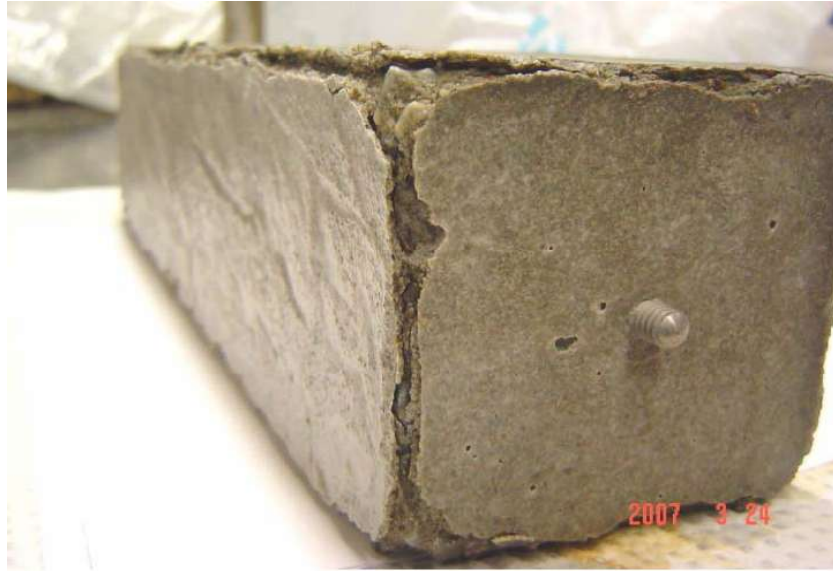
Figure 49. Photographs of concrete prisms subjected to 133 freezing and thawing cycles in 15% \text{CaCl}_2 solution.
