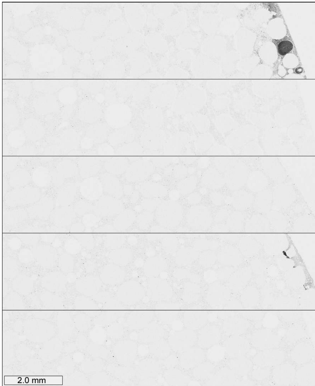
Figure 21. Elemental map for magnesium collected from thin sections prepared from mortar cylinders immersed in chemical solutions.
