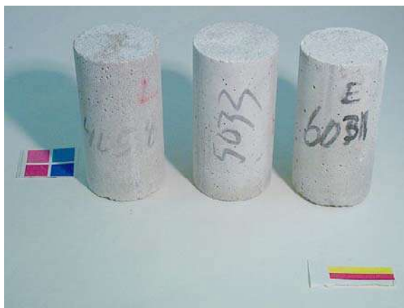
Figure 17. Control cylinders exposed to lime water solution after 84 days of constant low temperature test. From left to right: 0.40, 0.50, and 0.60 w/c mortar cylinders.
