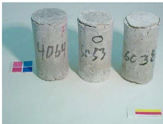
Figure 14. Cylinders exposed to MgCl 2 solution after 84 days of constant low temperature test. From left to right: 0.40, 0.50, and 0.60 w/c mortar cylinders.
