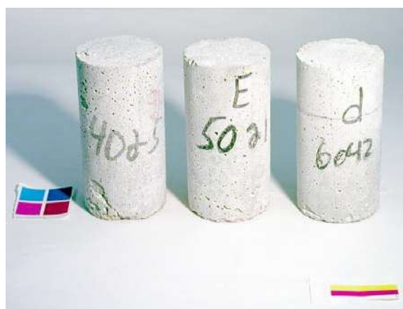
Figure 16. Cylinders exposed to CMA solution after 84 days of constant low temperature test. From left to right: 0.40, 0.50, and 0.60 w/c mortar cylinders.
