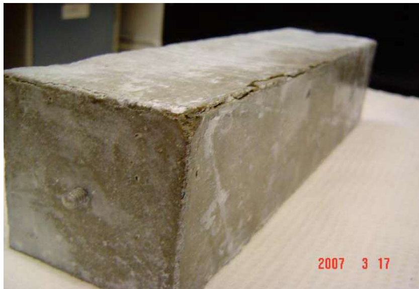
Figure 50. Photographs of concrete prisms subjected to 133 freezing and thawing cycles in 14% \text{MgCl}_2 solution.
