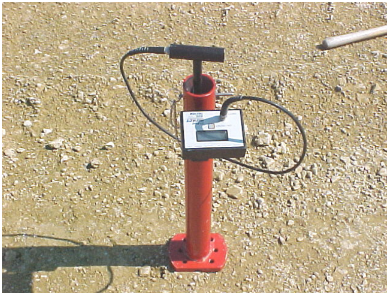
Figure 12. Clegg Impact Hammer
