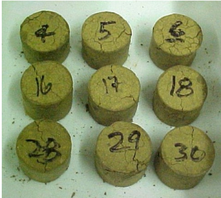
Figure 62. Swelling and cracking after soaking of paleosol and fly ash cured at 8° F
