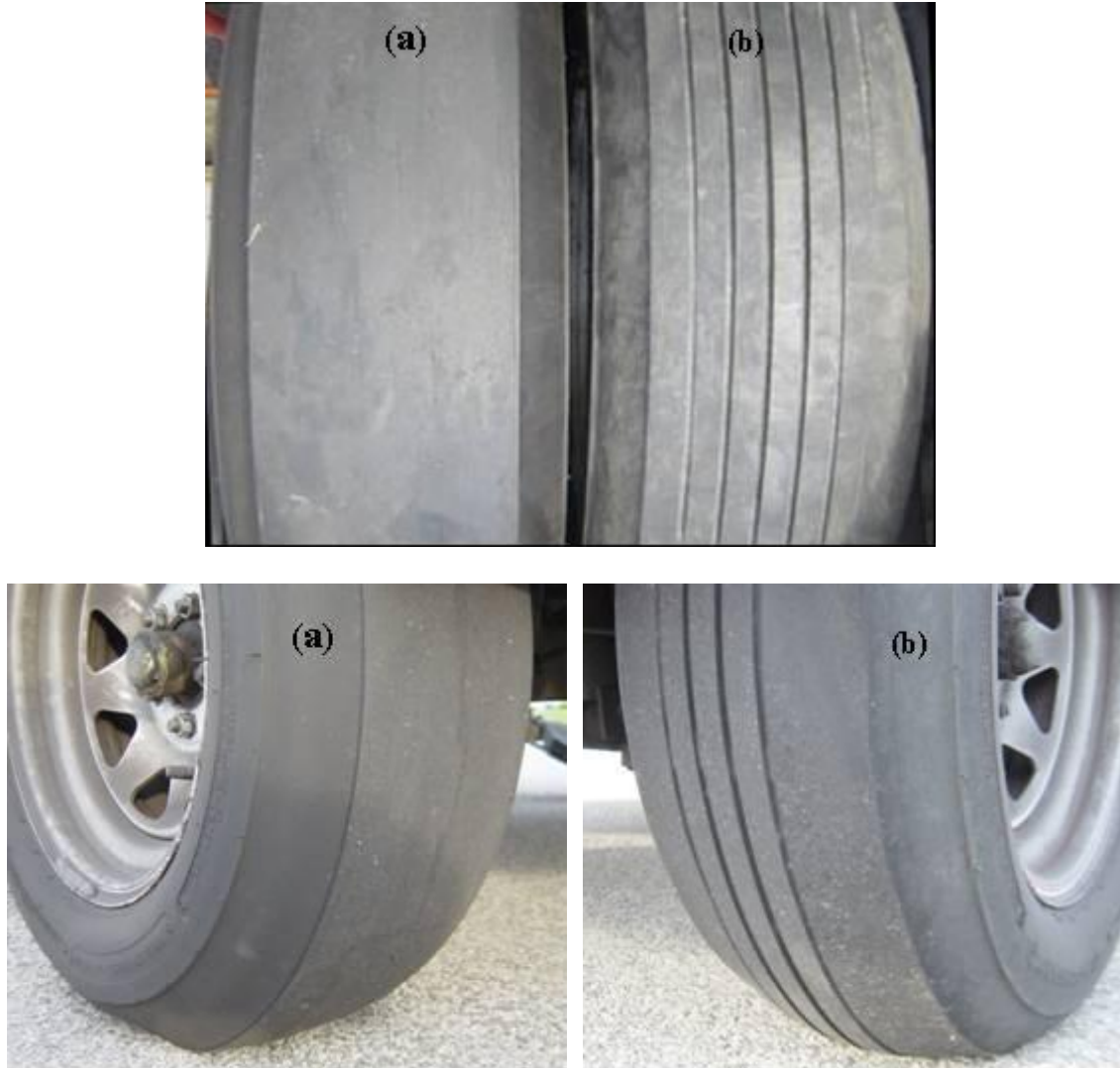
Figure 23. Tires used for the friction measurements: (a) smooth and (b) rib
