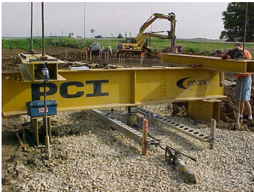
Figure 30. Geopier Field Modulus Load Test
