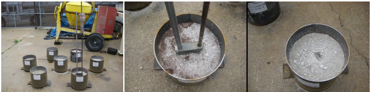
Figure 36. DCP testing on dry specimens after seven days
