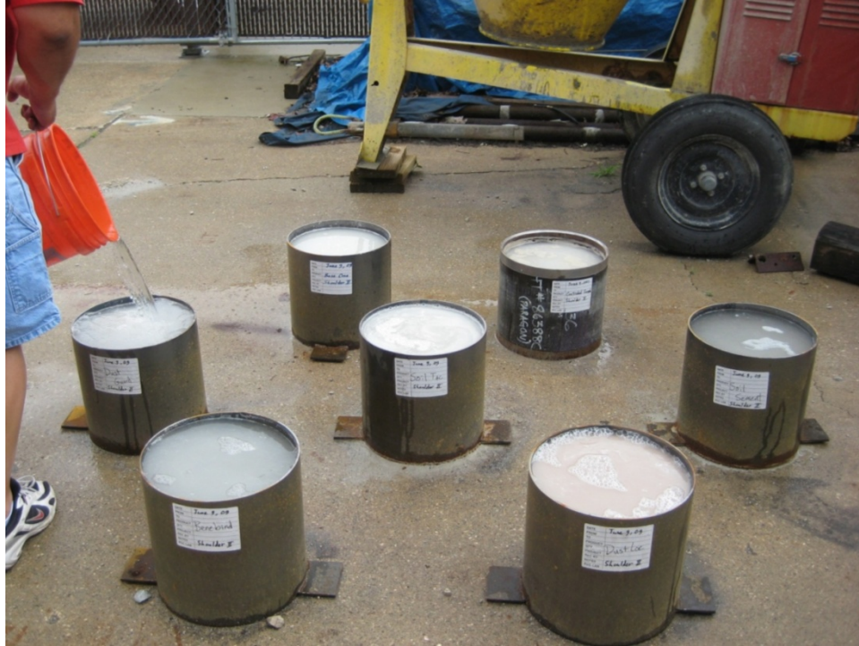
Figure 37. Specimens are saturated and kept three days for DCP testing in saturated conditions
