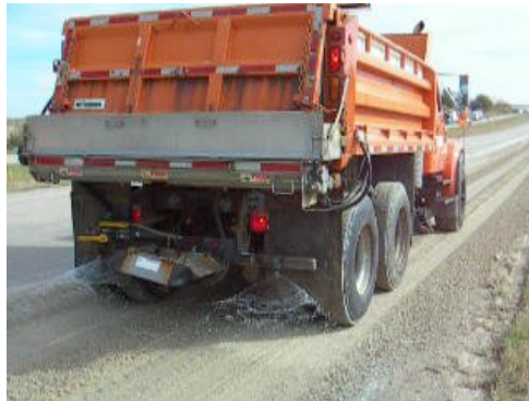
Figure 13. Dump body brine truck spraying Base 1 solution
