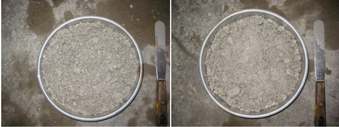
Figure 28. Mixtures of: a) aggregate and Soiltac and b) aggregate and diluted Soiltac
