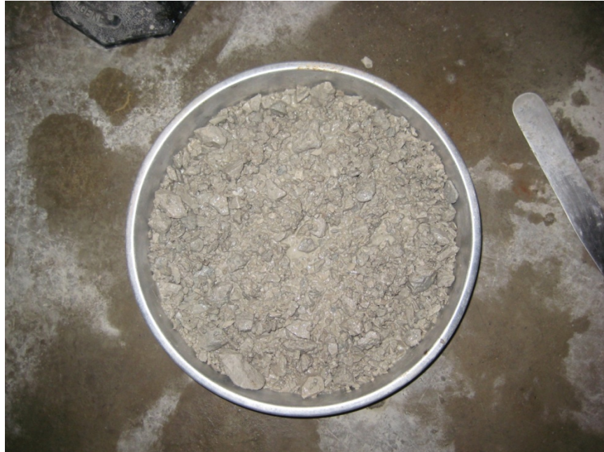
Figure 27. Mixture of aggregate and diluted Base One
