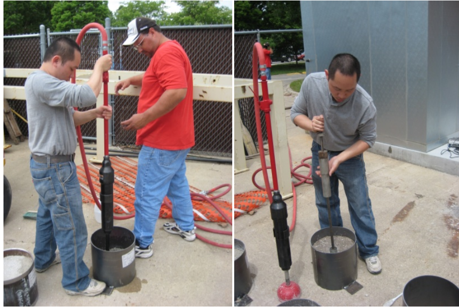
Figure 34. Specimen compaction: a) air compactor and b) surface finishing with the Marshall hammer
