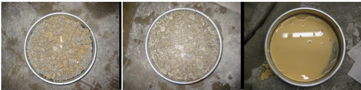
Figure 29. Mixtures of: a) aggregate and BENEbind, b) aggregate and diluted BENEbind, and c) diluted BENEbind
