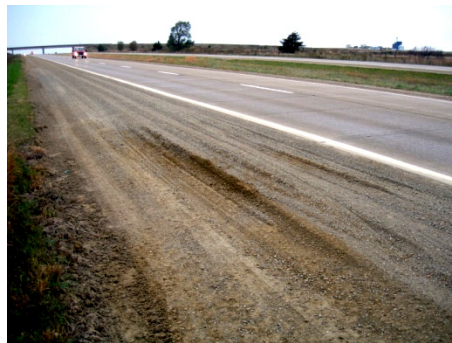
Figure 18. No stabilizer, full-depth, still soft one week later
