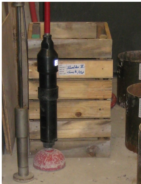
Figure 32. Wooden frame to protect the compactor from jumping out of compaction mold
