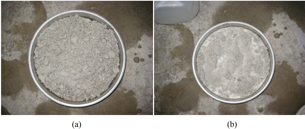
Figure 26. a) Mixture of aggregate and Soil-Sement and b) Mixture of aggregate and diluted Soil-Sement
