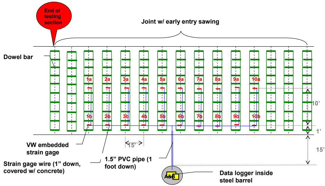
(a) Part I – Early entry sawing
