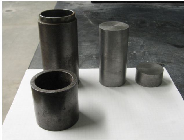
Figure 9. Mold apparatuses for static compaction
