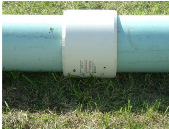
Figure 4.124. Certa-Lok ® bell (16-inch diameter) connecting pipe sections (12-inch diameter)
