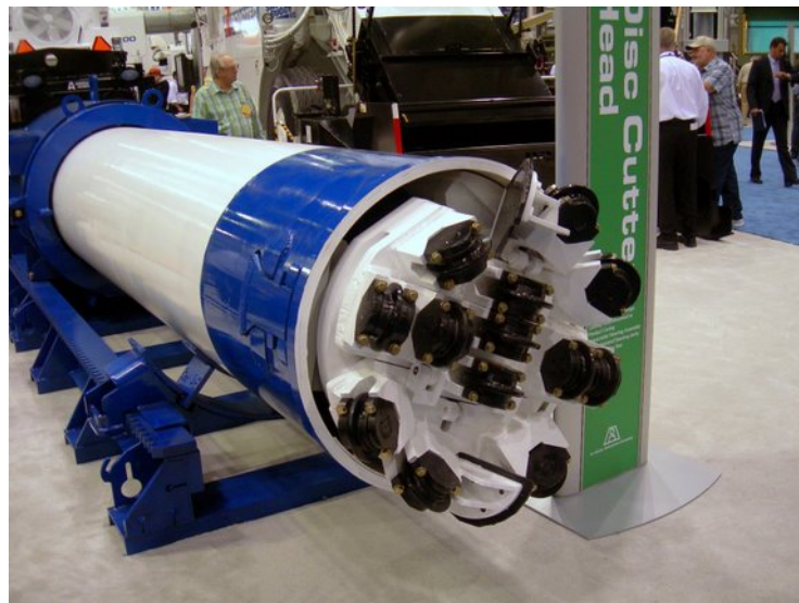
Figure 2.8. MTMB with disc cutter head on display (photo by Charles T. Jahren)
