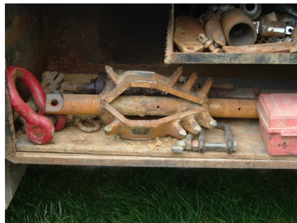
Figure D.23. Fourteen inch diameter reamer
