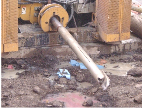
Figure 4.76. Pilot bore drill bit attached to drill rig
