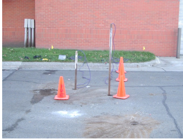
Figure 4.82. Push-in pressure cells in place at point B (looking south)
