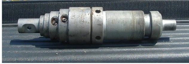
Figure 4.109. Grundomat reciprocating stepped-cone chisel head
