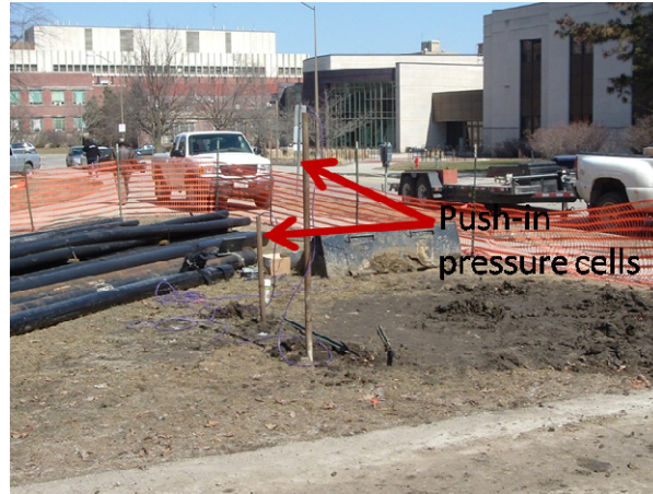
Figure 4.88. Push-in pressure cell after installation
