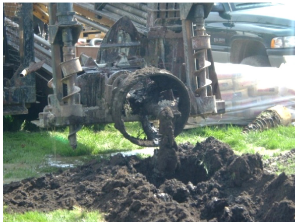
Figure D.46. Twenty-four inch wagon wheel reamer
