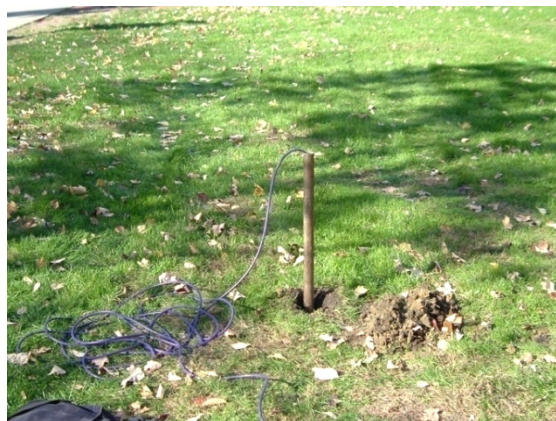
Figure 4.66. Push-in pressure cell after installation
