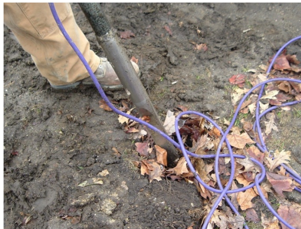
Figure 4.91. Push-in pressure cells being removed
