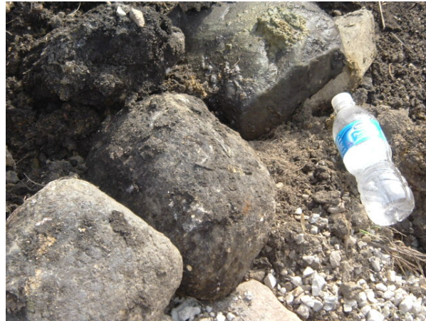
Figure 4.23. Boulders removed from the borehole (12 to 18 inches in diameter)
