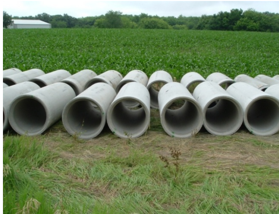
Figure D.4. Twenty four inch concrete pipe
