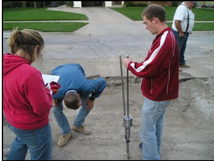
Figure 5.19. Dynamic cone penetration test being performed in Trench BI
