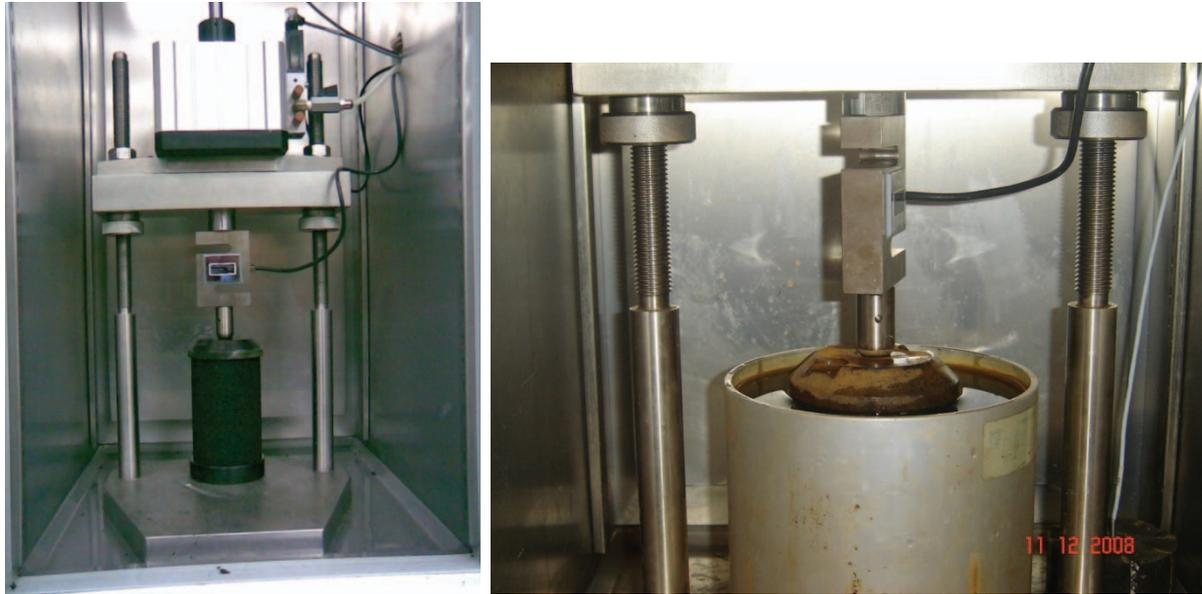
**Figure 3-2. Flow number test setup**
