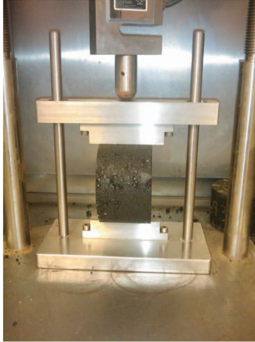
**Figure 3-3. Indirect tensile strength test setup**
