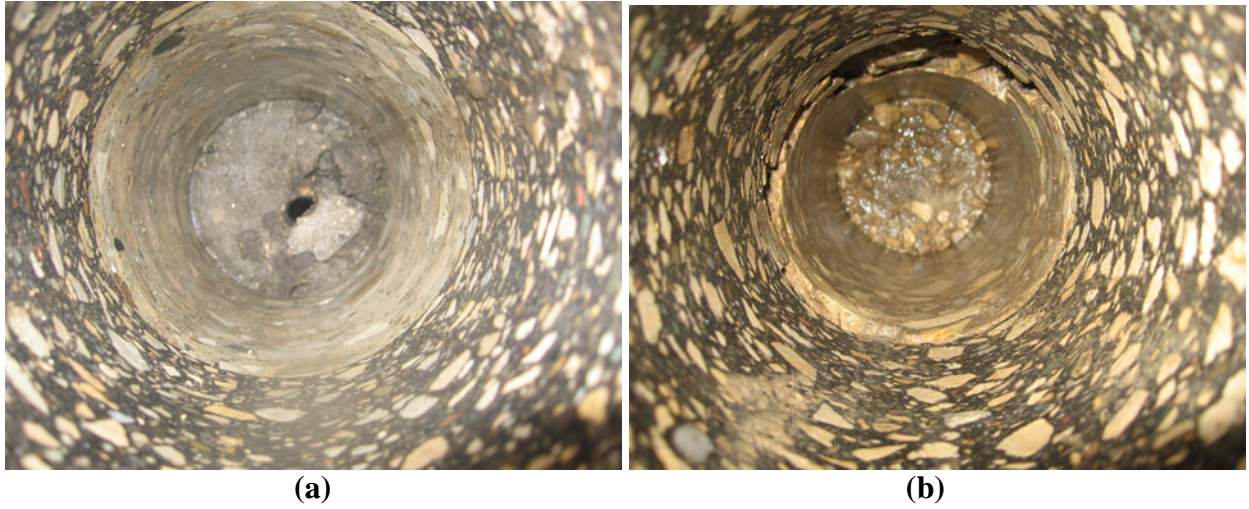
Figure 7. Layer condition underneath HMA after coring; (a) PCC layer without rubblization (IA-139 in Winneshiek County), (b) Rubblized PCC layer (IA-3 in Delaware County)
