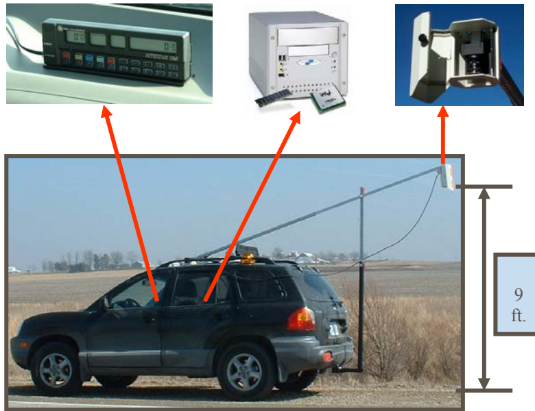
(a) Configuration of automated image collection system
