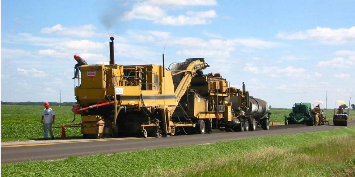
Figure 2. Picture of a typical CIR recycling train
