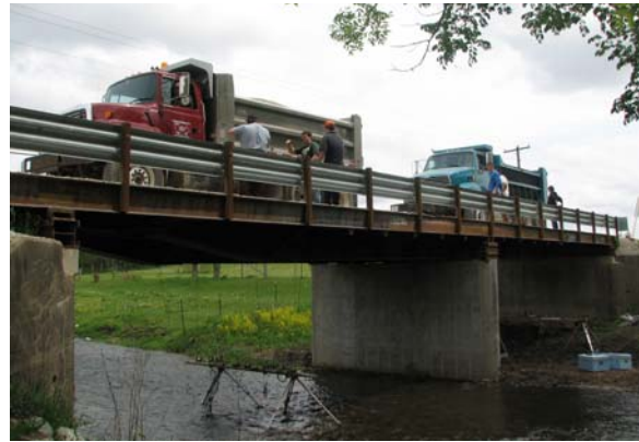
b. Side view of two-truck load test
