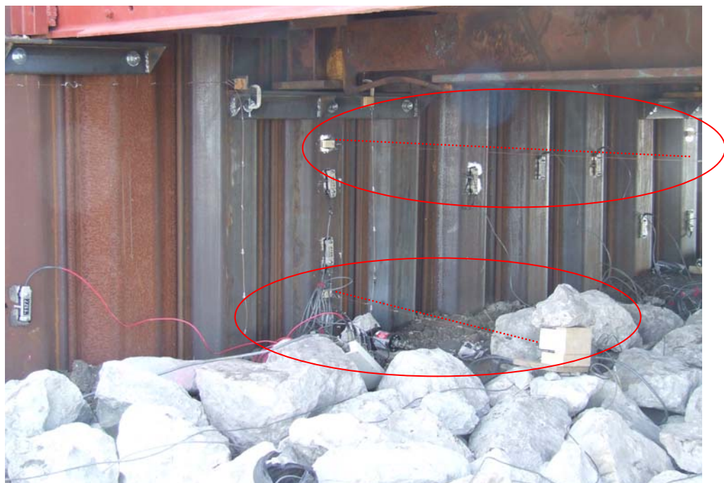
Figure B.12. Instrumentation measuring displacement in the direction of the bridge
