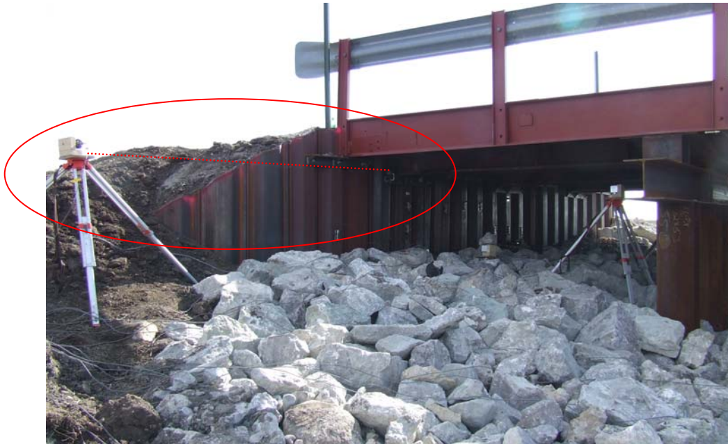
Figure B.11. Instrumentation measuring displacement perpendicular to traffic
