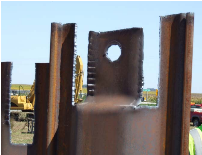
Figure B.5. Buckled sheet pile section due to driving equipment
