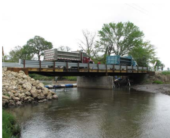
a. Side view of two-truck load test
