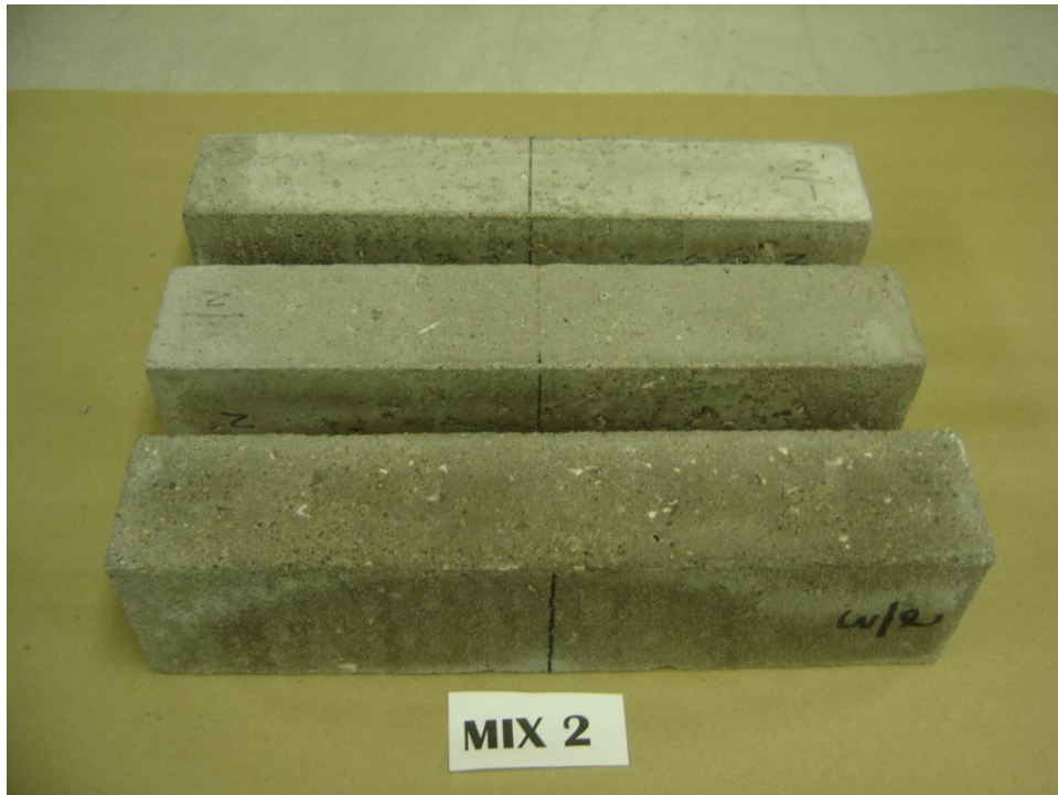
Figure 4 – Freeze thaw beams – Mix 2
