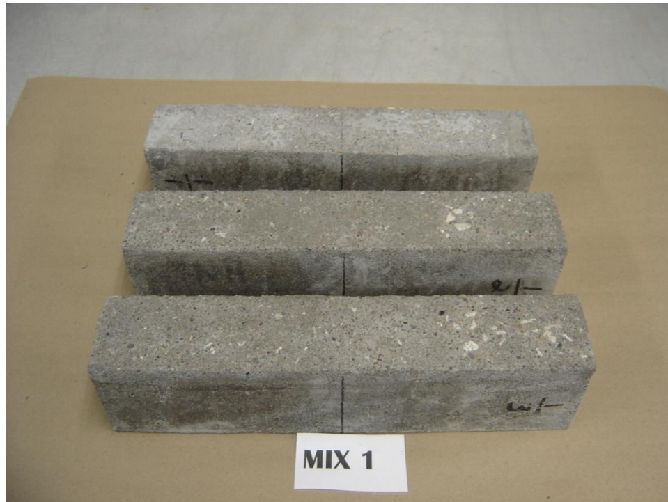
Figure 3 – Freeze thaw beams – Mix 1
