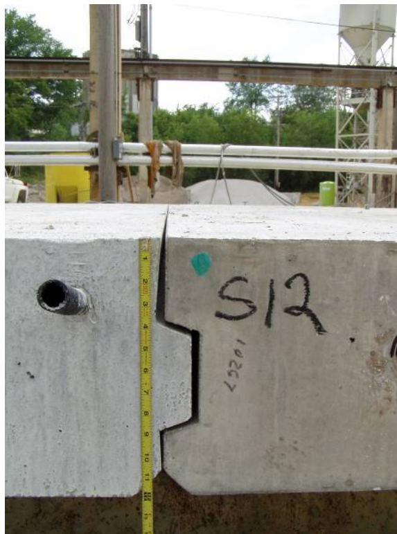
Figure 22. Battered keyway after removal from forms.
