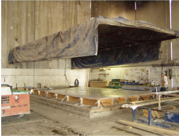
Figure 17. Curing tent being lowered to cover a precast panel after casting.
