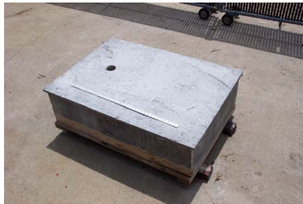
Figure 3. Slab containing crossed reinforcing bars (3/8-inch nominal diameter)
