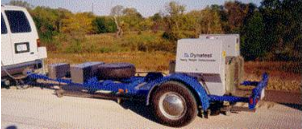
Figure 3. Falling Weight Deflectometer
