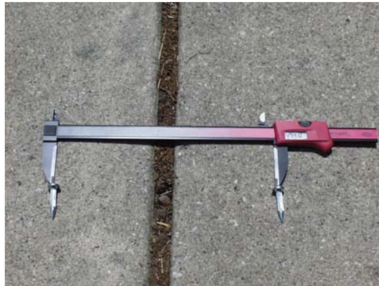
Figure 5. Calipers and Surveyor Nails (Nails Not Installed)
