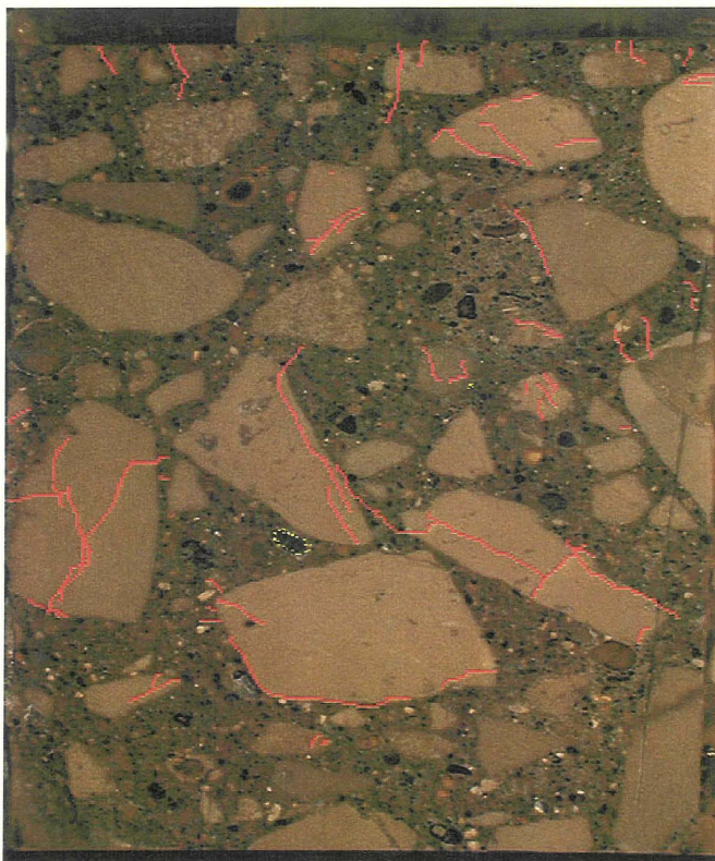
Figure 16. Cracking (red) and ASR (yellow) in Core 7 as observed using SEM. Cracking of aggregate is common. Surface cracks appear carbonated and terminate in both the mortar and the coarse aggregate. Micrograph field width is approximately 10 cm.
