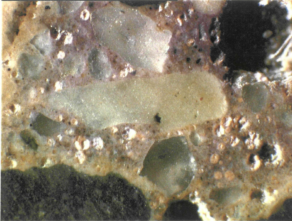
Figure 11. Iowa 175 Core 2 base mortar microstructure exhibiting partial filling of the entrained air void system. Micrograph field width: 4 mm
