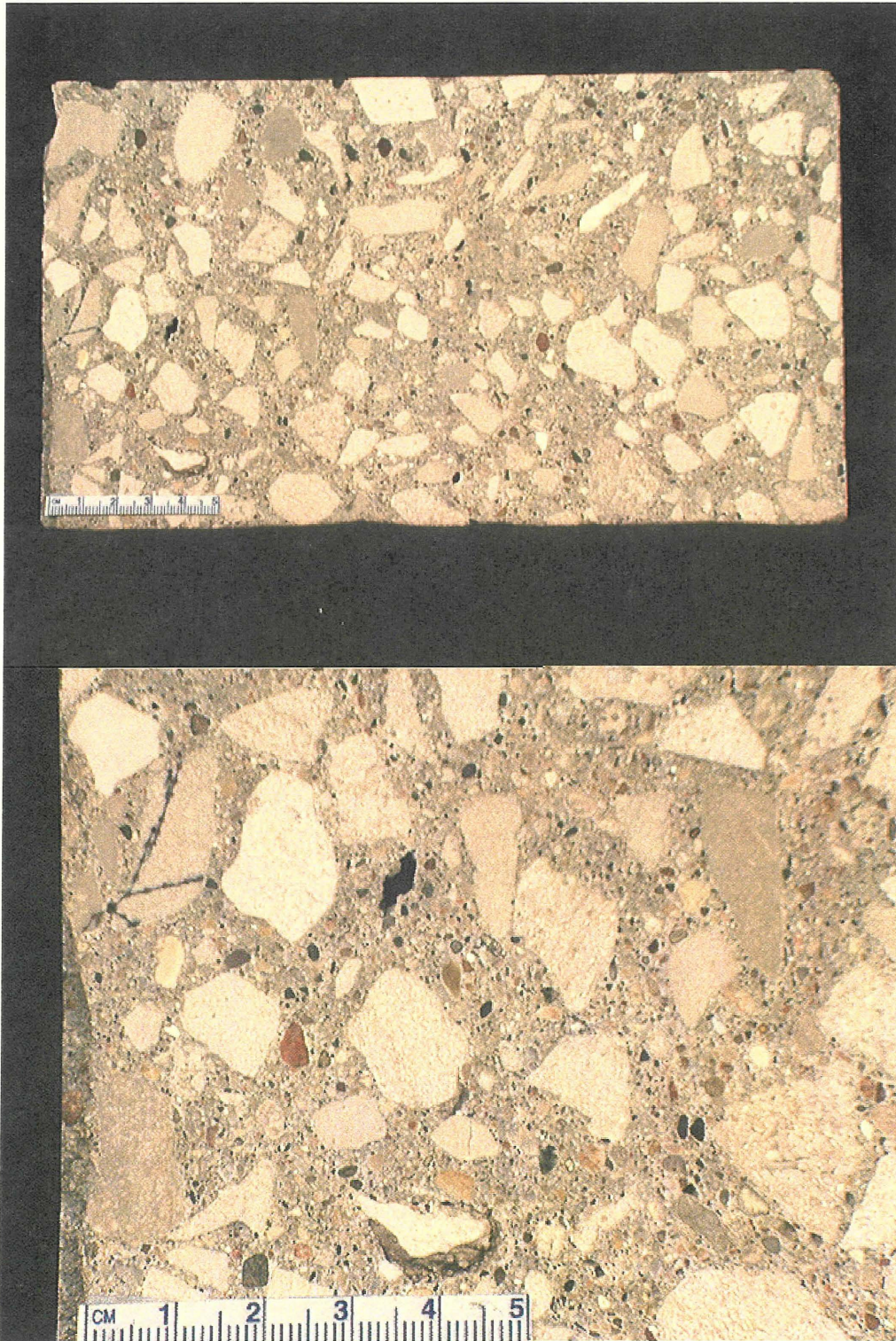
Figure 21. Core 14 exhibits some cracking of both the paste and coarse aggregate and some mortar / aggregate segregation in middle.
