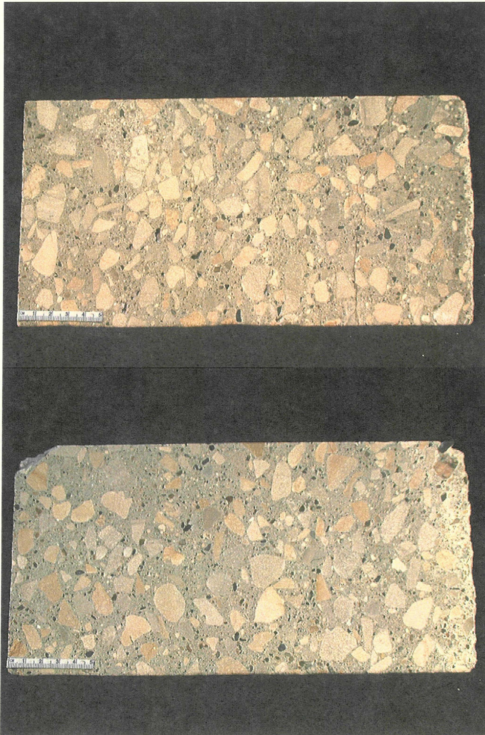
Figure 38. Cores 11, joint (top) and 12, mid-panel (bottom) cross section with horizontal crack in lower-most third. Some segregation is visible in both cores.
