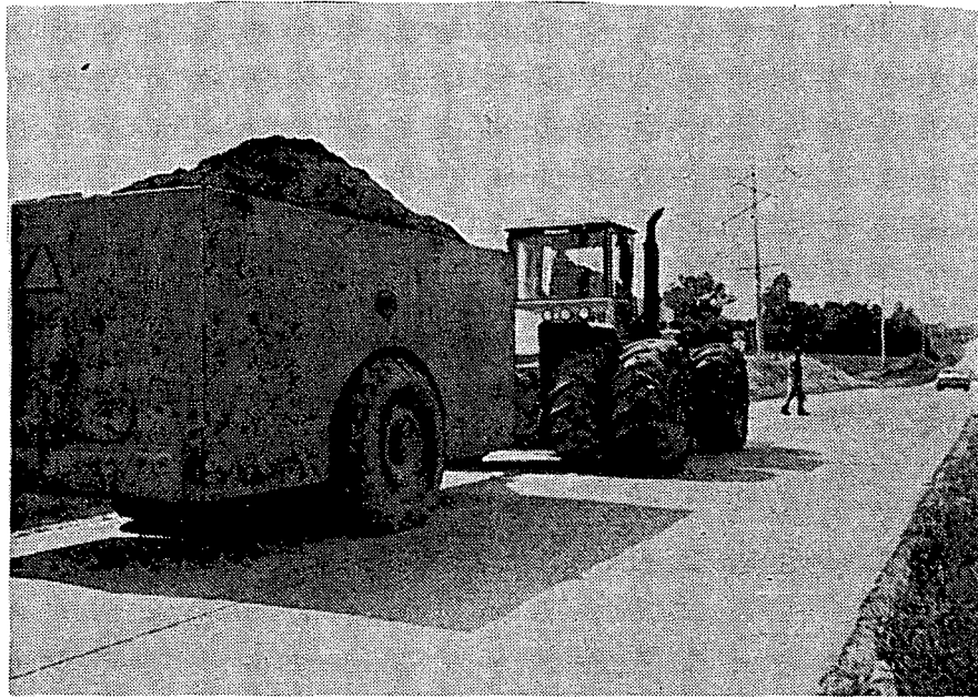
Figure 3 - Bros Proof Roller Used For Seating
