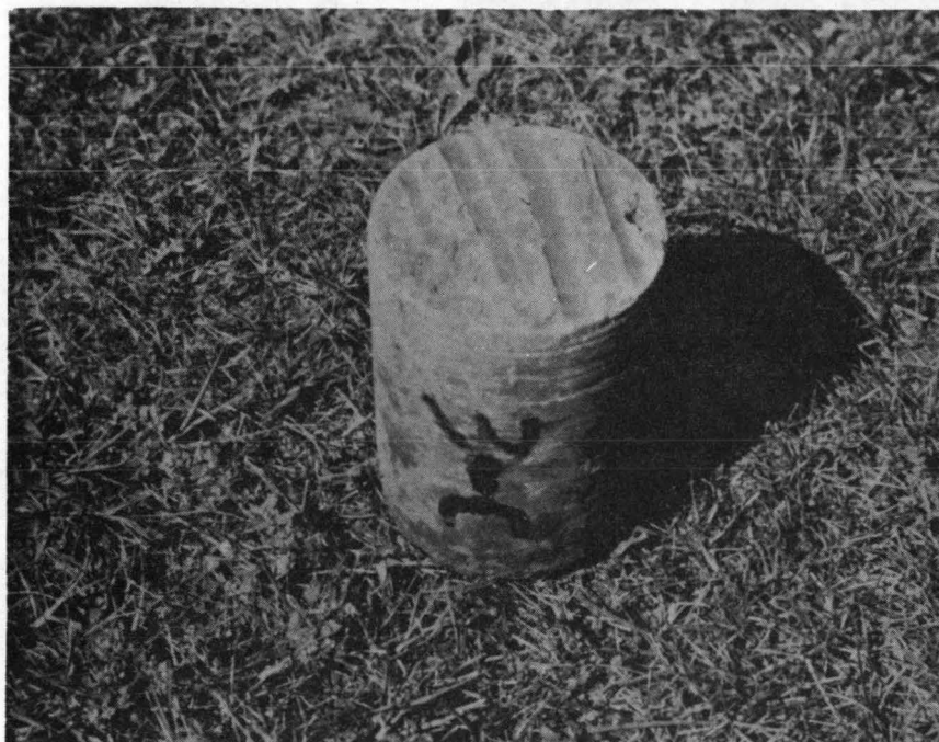
PHOTO 26: Core sample from soil-cement base. Note marks caused by the spike-tooth drag. During coring operations the core broke on this plane ( \frac{1}{2} to 1" below surface).
