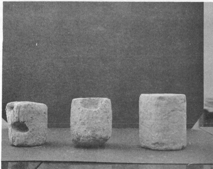
PHOTO 25: Core samples after completion of 12 freeze-thaw cycles. Note the voids in the two cores on the left due to disintegration of clay lumps present in the mix.
