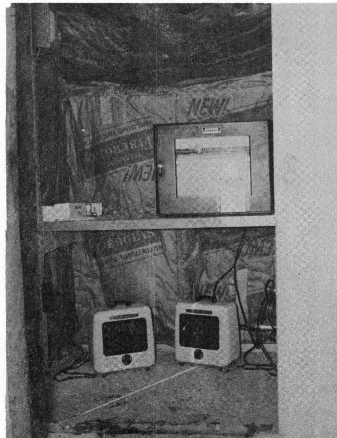
PHOTO 29: Interior of temperature recording installation. Recording potentiometer (upper right), thermostatically controlled space heaters (below).
