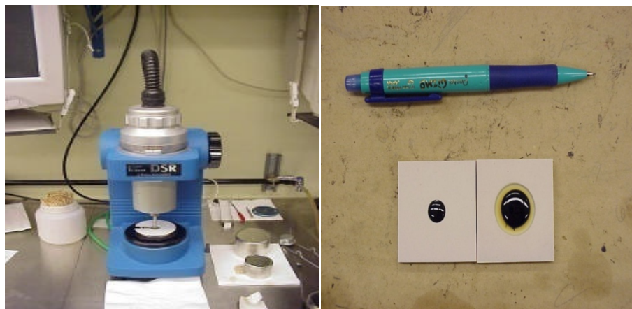
Figure 3.9. Dynamic Shear Rheometer Machine and the Sample
