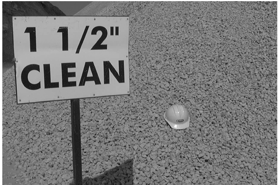
Broken concrete is recycled and reused at Corell Recycling
