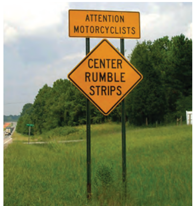
Figure 4.16. CLRS advance warning (Chatham County, Georgia Signs 2009)
