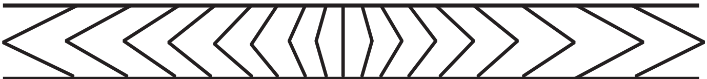
Figure 6.15. Wundt-Herring pavement marking layout (Shinar et al. 1980 and Godley 1999)
