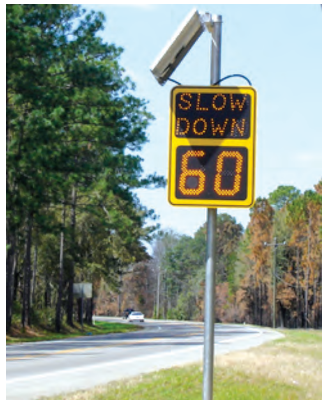
Figure 6.9. Speed-activated signs in Ohio and Florida (top: Hawkins, InTrans)
