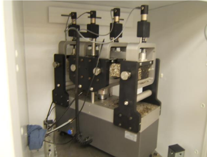
Figure 1. Iowa State University's four-point bending beam
