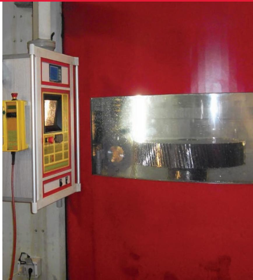
**Left:** A gear blank being turned on PEM's You Ji Vertical Lathe by machinist Brian Oman. **Right:** PEM's Hofler Rapid 2000 Geargrinder cutting teeth into the gear blank.
