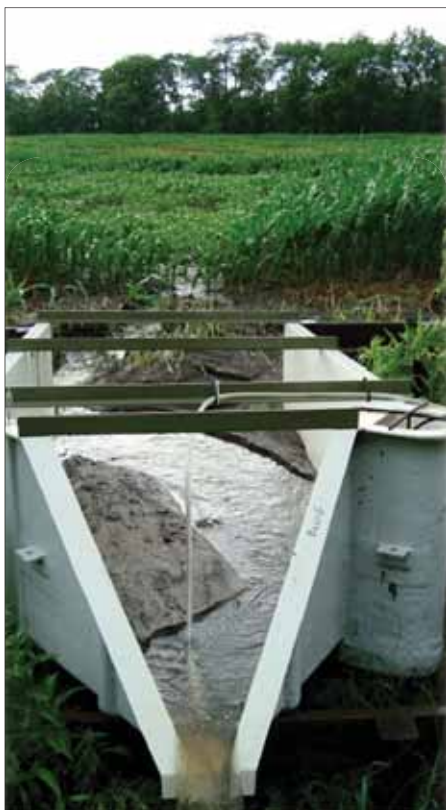
This flume collects field runoff from research plots at the Neal Smith National Wildlife Refuge.
