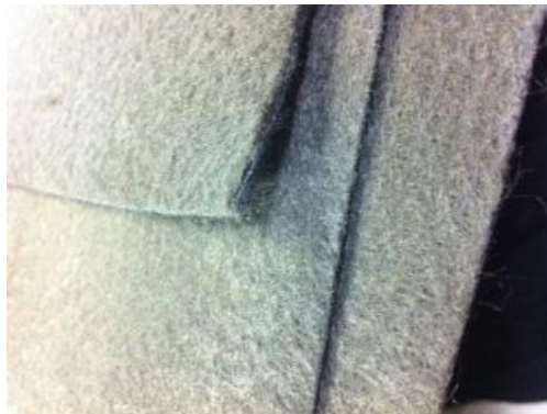
Figure 26. Non-Woven geotextile (Photo courtesy of Propex Infrastructure Solutions)
