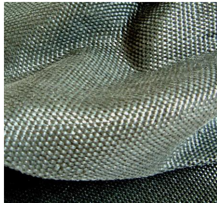
Figure 27. Woven geotextile (Photo courtesy of Propex Infrastructure Solutions)
