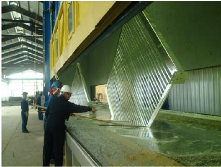
Figure 2-4. Steel dipped into molten zinc bath [16] ( www.zinc.org )
