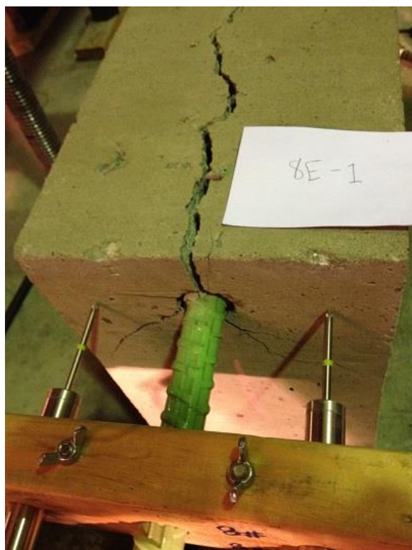
(a) Specimen with #8 epoxy-coated test bar
