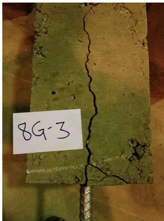
(b) Specimen with #8 galvanized test bar
