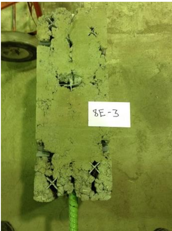
(c) Specimen with poor concrete consolidation
