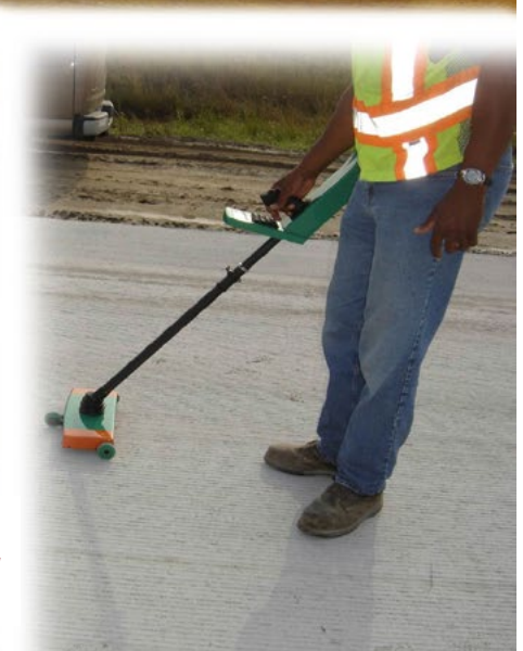
The Iowa DOT is using the MIT-SCAN-T2 device for determination of concrete pavement thickness to replace the traditional coring method.
