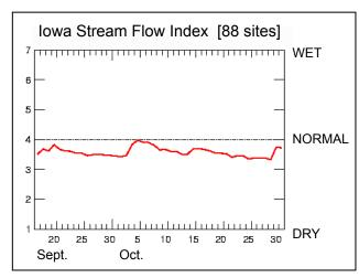
This chart provided by the U.S. Geological Survey shows the increased average stream flow that occurred as a result of recent rain.
