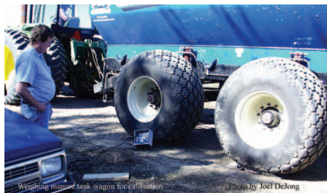
Weighing manure tank wagon for calibration
