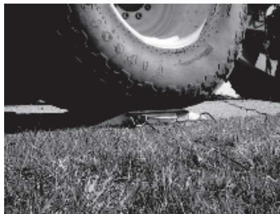
Weigh-pad used to weigh manure tank wagon.
