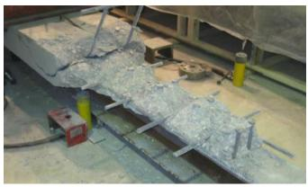
Second peeling test (2 shear studs) (Dahlberg 2014)
