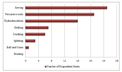
Currently allowed deck removal methods for steel I-girders
