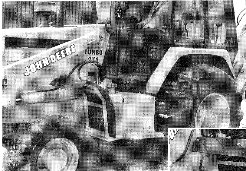
Mud flaps on the front wheel of this tractor prevents mud from obscuring the driver's vision. The inset photo shows how the mud flap is attached to the tractor.
