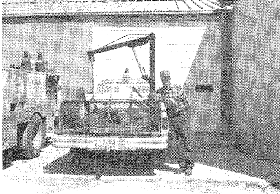
Fremont County mechanic Rich Barrett with his "homemade" pickup mounted hoist.
