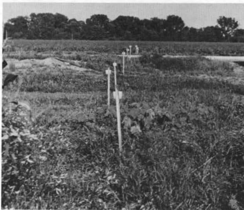
Fig. 6. Road dust collectors installed at 20 ft intervals up to 140 ft each side of center-line.
