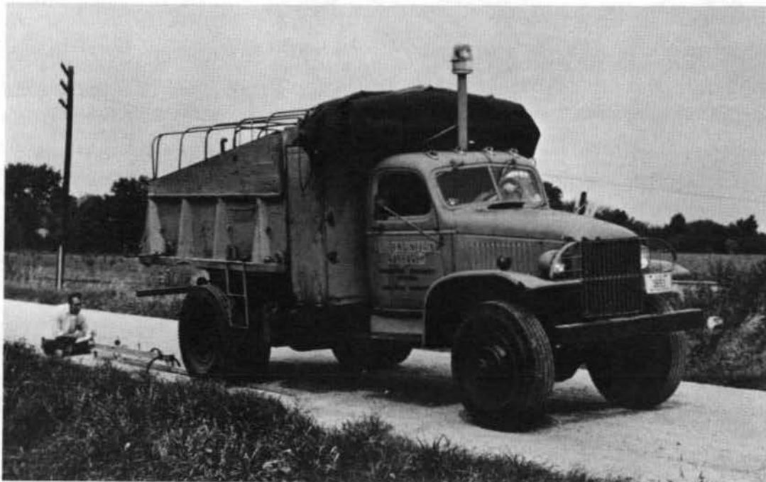
Fig. 24. Benkelman beam deflection test in process.
