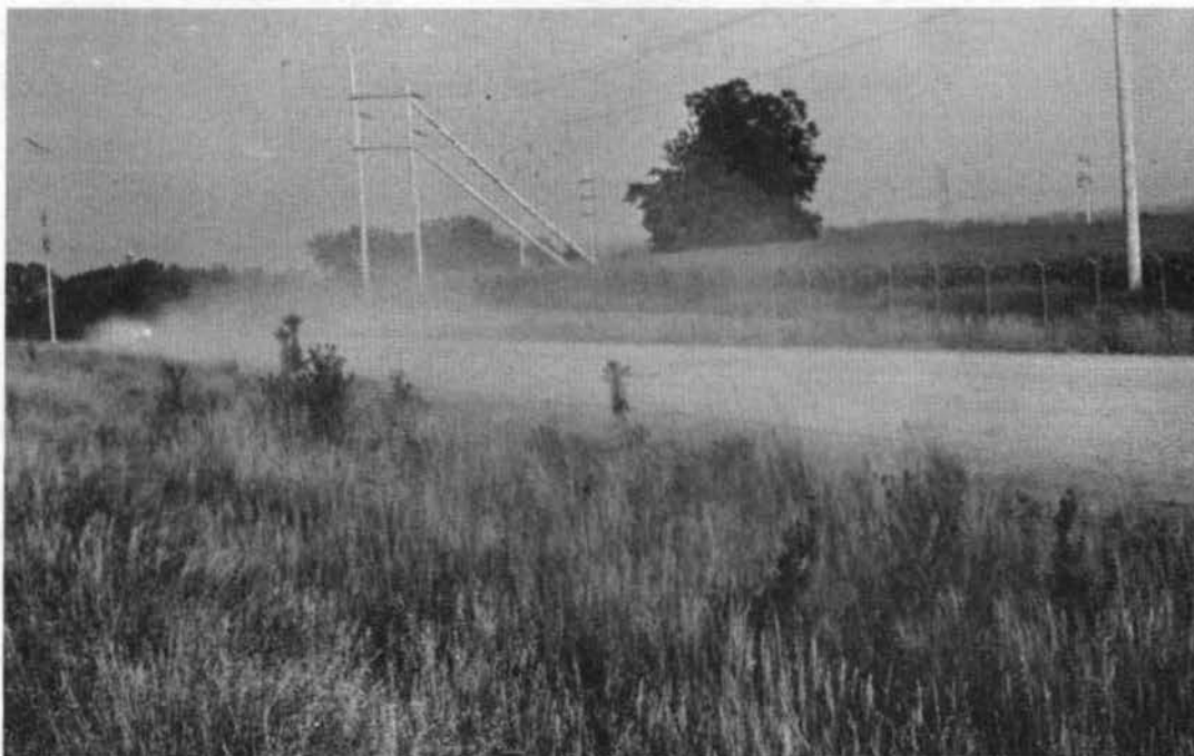
Fig. 20. Clinton county, residual test section dust prior to treatment. Vehicle speed, 40 mph.
