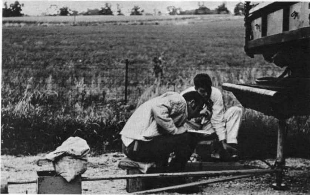
Fig. 23. Spherical Bearing Value (SBV) test in process.
