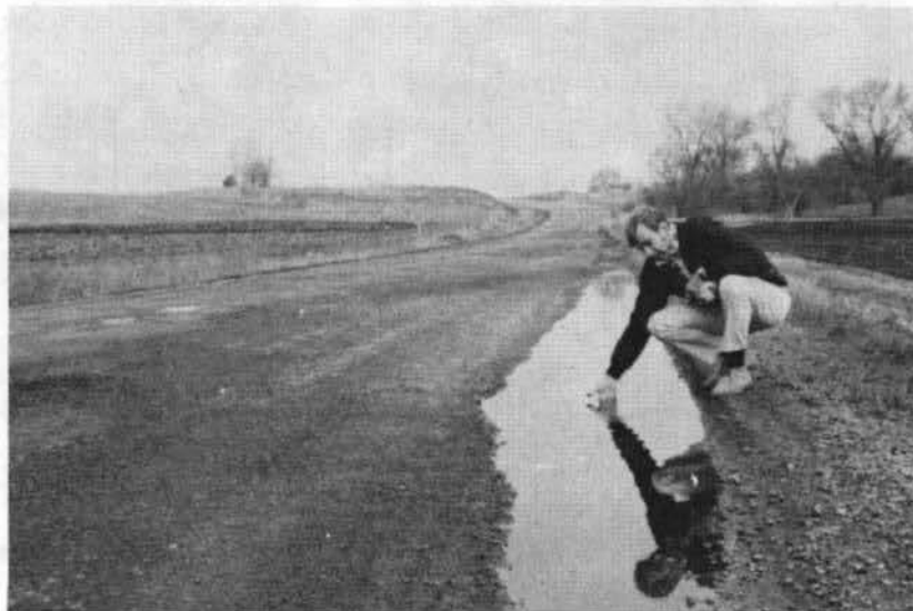
Fig. III-41. Rutting, 1% lignosulfonate plus 0.5% lime additive section, looking north, spring 1971, Clinton test road.
