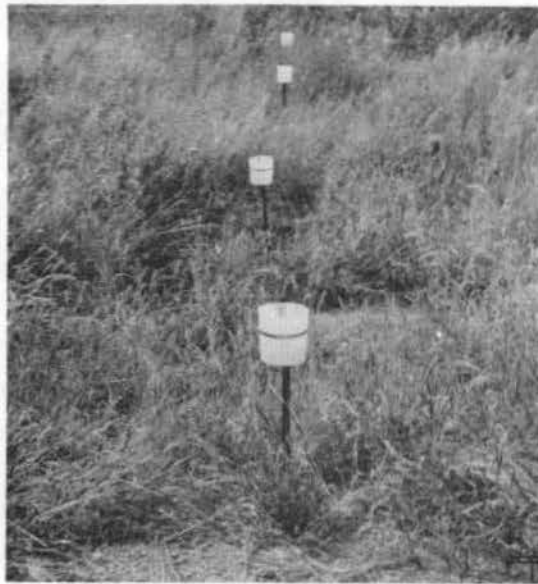
Fig. III-47. Dust collectors, summer 1971, Marion test road.
