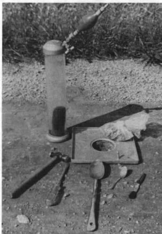
Fig. III-32. In-place balloon density apparatus.
