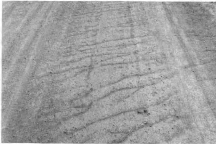
Fig. III-42. Surface runoff channels, 1% lignosulfonate additive section, spring 1971, Clinton test road.
