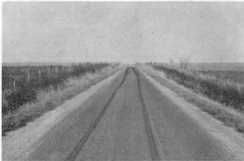
Fig. III-53. Lignosulfonate dispersed surface after drizzle on 2% lignosulfonate, low aggregate content, section 1, October 1971, Marion test road.
