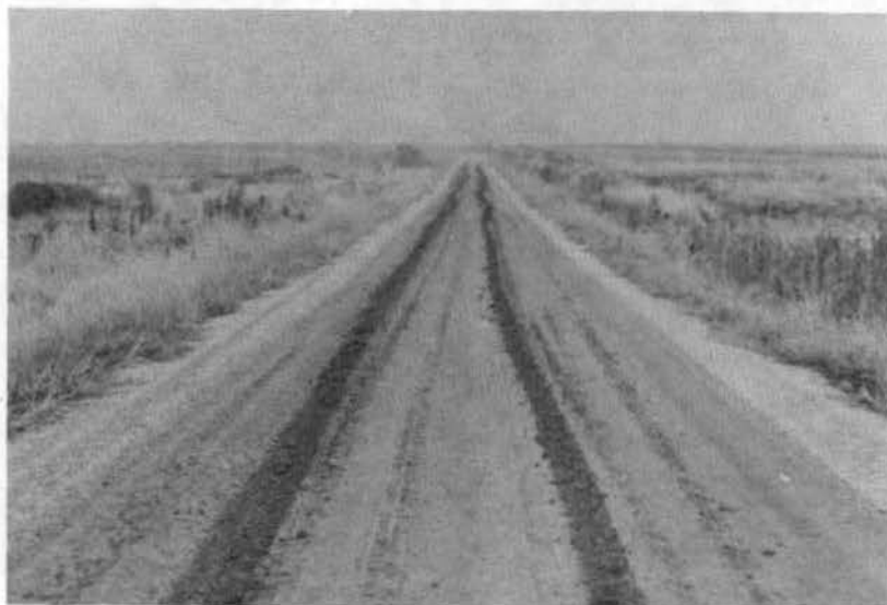
Fig. III-52. Lignosulfonate dispersed surface after drizzle on low and intermediate aggregate content sections, October 1971, Marion test road.
