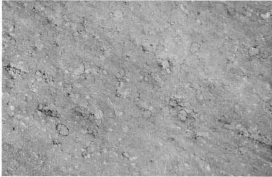
Fig. II-36. Mudballs in MC-800 sections 1 and 2 (4% residual asphalt).
